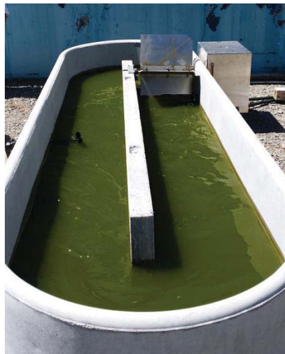
Figure 3.9: 1000 L HRAP fed primary wastewater
