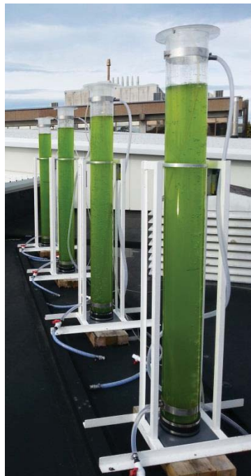
Figure 3.1: C. vulgaris cultivated in 50 L bubble column photobioreactors (2 m × 0.19 m inner diameter, 1 m 2 of illuminated area as described by Béchet et al. (2010)).
