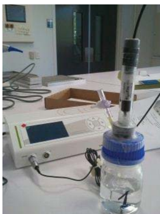
Figure Q.1: Set-up used to measure dissolved N 2 O with Unisense N 2 O microsensor.
