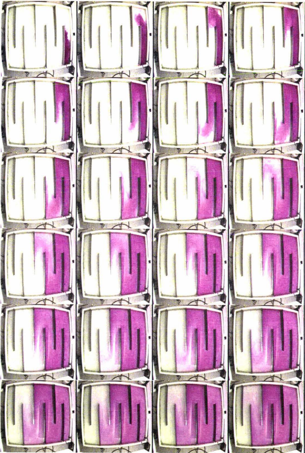
Figure 5-6 Dye Flow Path - Lab Tracer Study Case L4 (traditional six baffle case)
