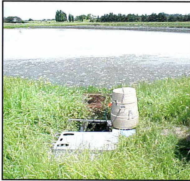
Figure 6-2 Auto-sampler set-up at outlet - Ashhurst pond
