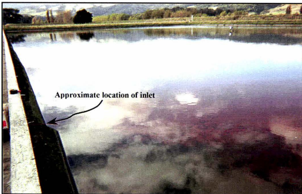
Figure 6-4 Dye movement - Ashhurst Field Trial 1
