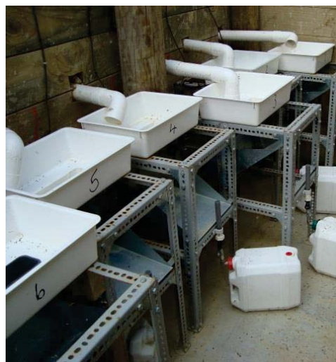
Figure 6.3. Photos of (A) the collection pit (A) and (B) tipping buckets and sample collection containers. Note that the stilling wells in the photo were removed prior to the trial commencing.
