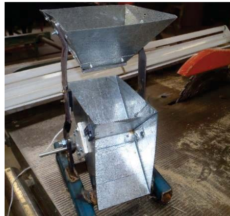
Figure 4.4. Photos of the sampling pits and tipping buckets in 2013. Photos are: A. sampling and drainage pit with drainage pipe connected, B. Altering the sampling pit to make it deeper, C. Tipping bucket in position in the sampling pit, D. Tipping bucket.
