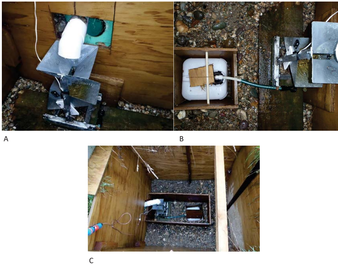
Figure 4.5. Photos of the enlarged sampling pits in 2014. Photos are: A. Pipe directing drainage into tipping bucket located in larger sampling pit, B. Composite sample container located below the base of the pit, C. View of the whole sampling pit.
