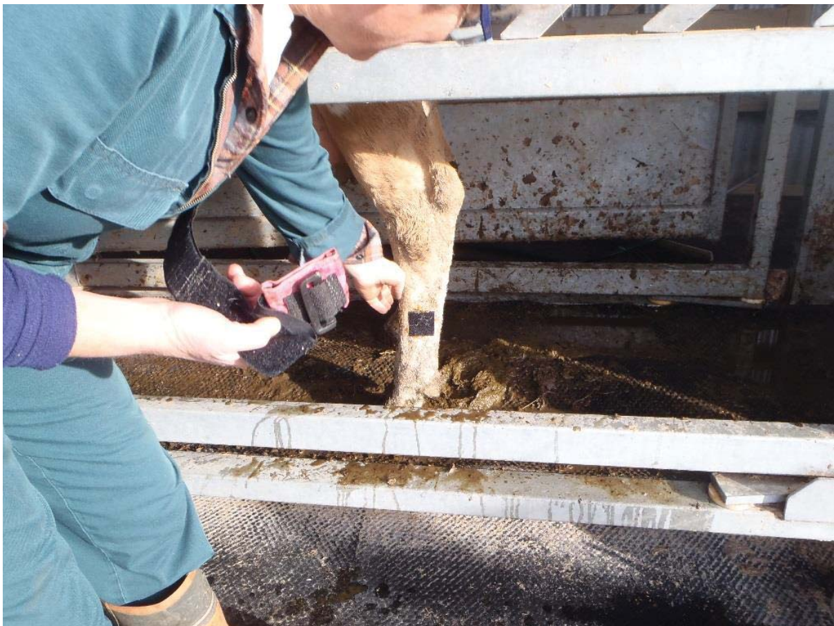
Figure 5.6. Attachment site for Hobo logger used to record cow lying times. The logger is housed in a pouch which is then attached to the leg by a strap and velcro (shown above).
