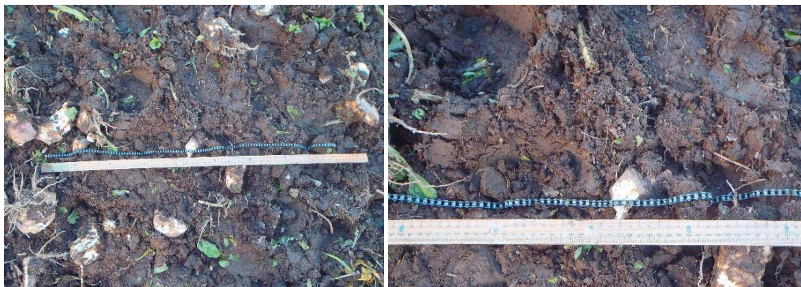
Figure 5.8. Chain measurement of determining a quantitative value for determining surface roughness for crop paddocks
