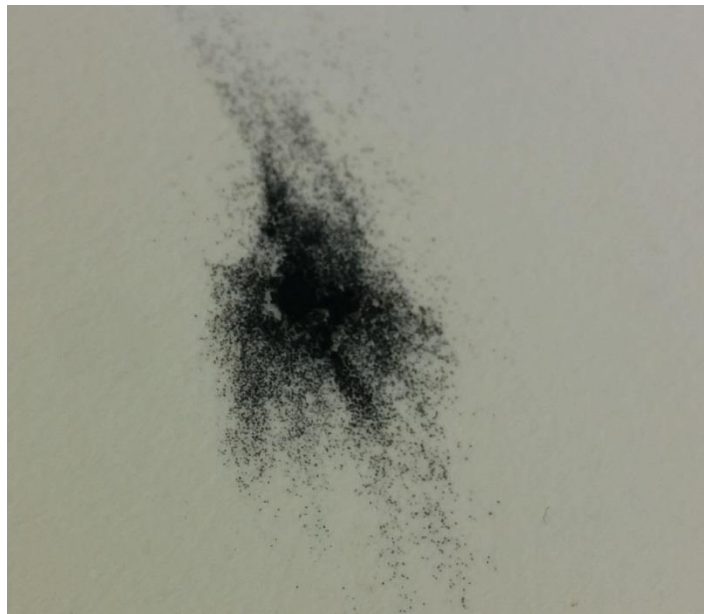
Figure 44 - Test with stationary print head showing inkjet overspray
