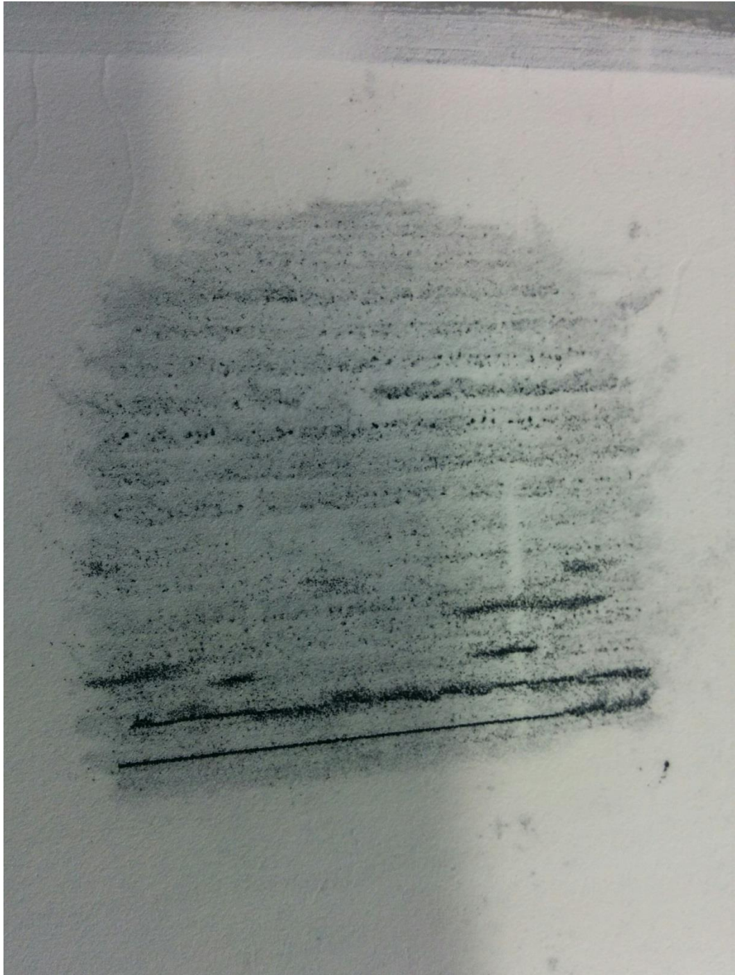
Figure 46 - Ink soaking through into a fresh layer of powder
