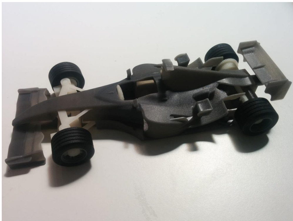
Figure 2 - Example of a part 3D printed in the in-house ProJet 5500X
