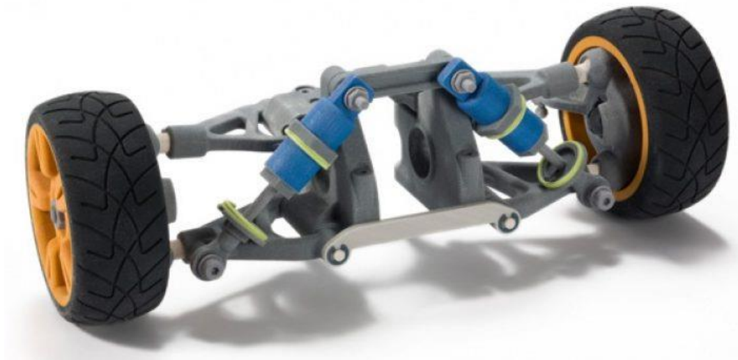
Figure 10 - Sample part 3D printed on the 3D Systems ProJet CJP 660Pro (DesignPoint, N.D.)
