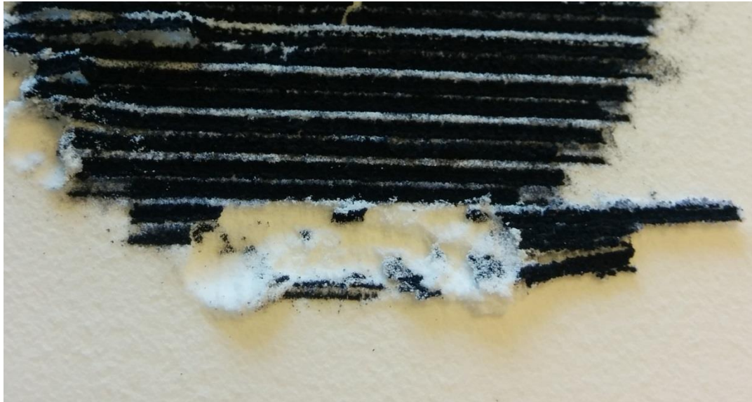
Figure 45 - Single printed layer partially bonded
