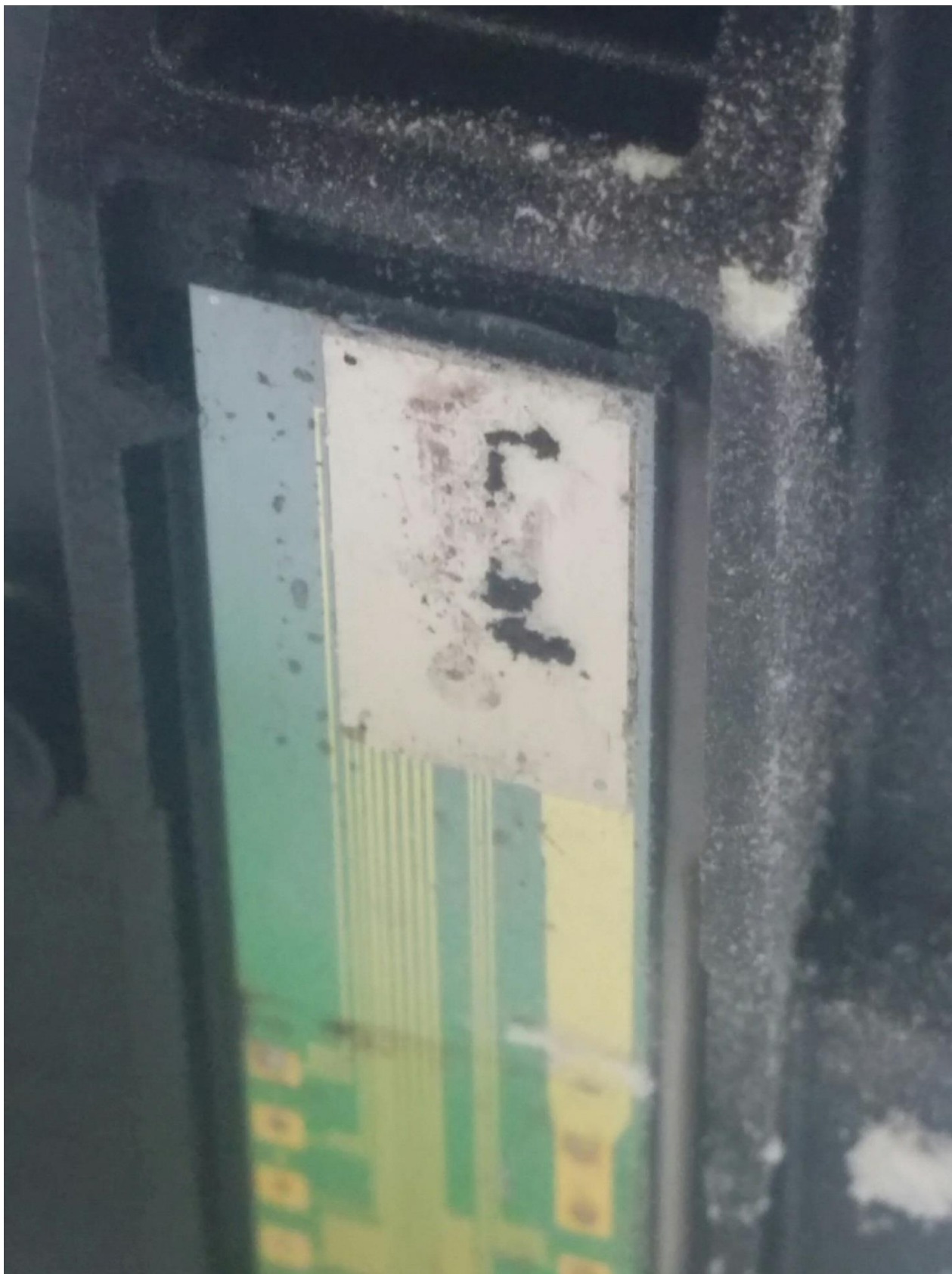
Figure 37 - Close up of the print head showing ink that has dried on the nozzle surface and powder stuck to the surface
