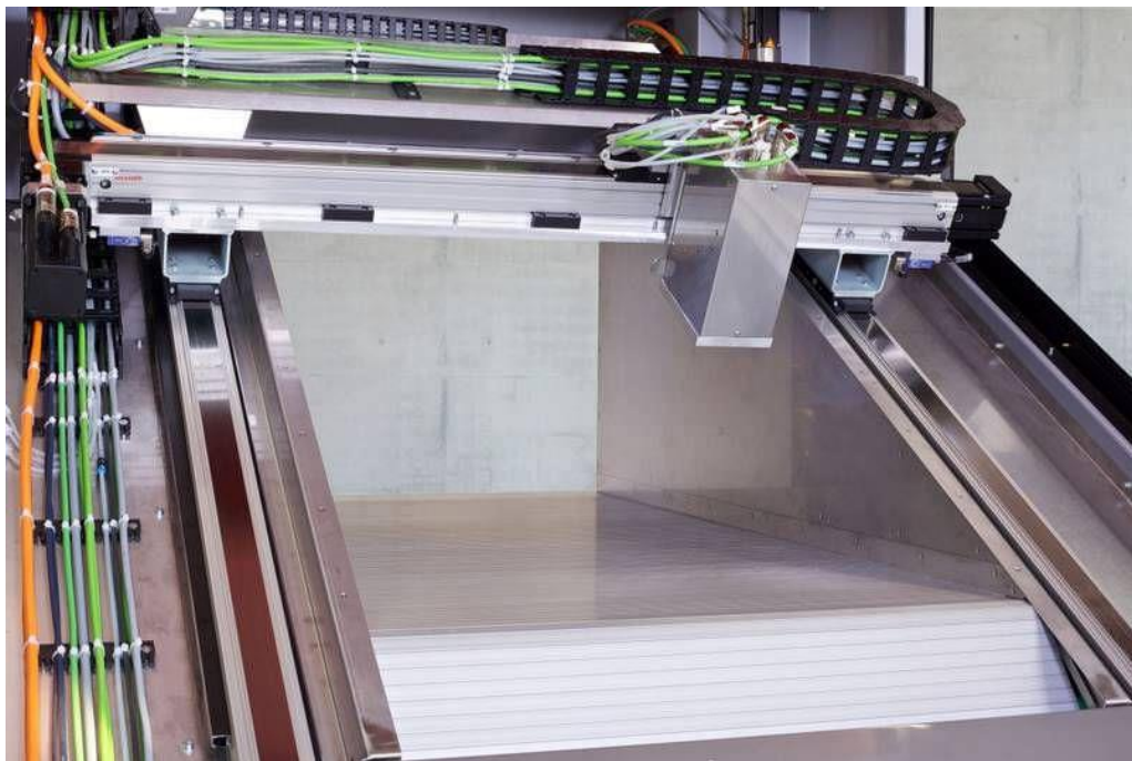
Figure 6 - View of the Voxeljet VXC800 angled print area and conveyor (3ders, 2012)
