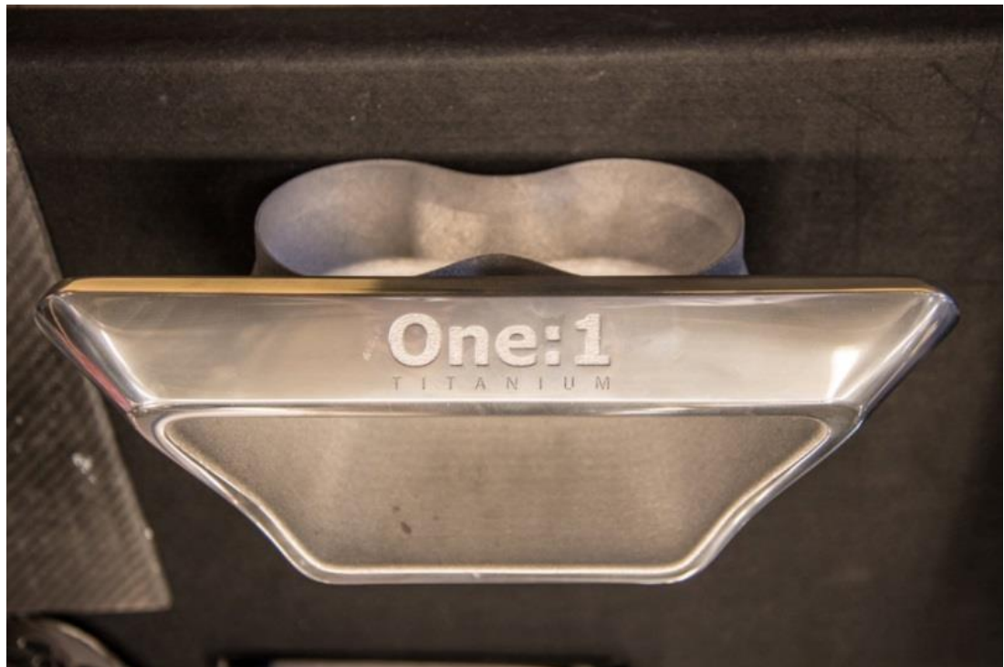
Figure 11 - Titanium 3D printed exhaust for the Koenigsegg One:1 (Wade, 2015)
