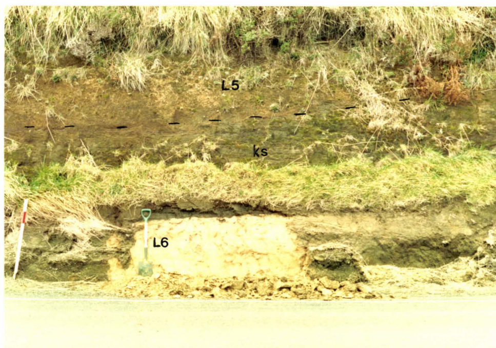
Plate 3.35 Sharp contact between L6 and the Kaihuahua dunesand (ks) which is c. 2 m thick, and is overlain by L5. Section 3 (Mangaroa Stream) at Q21/318678. Spade for scale is 1 m long.
