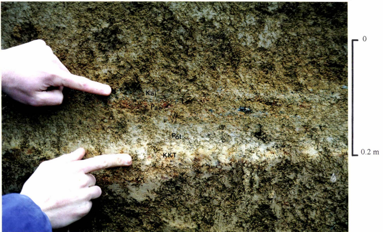
Plate 3.11 Medium to coarse grey and yellow/red lapilli of the Kaihouri Tephra (Kai) overlying medium yellow/red lapilli of the Paetahi Tephra (Pae). Fine grey/brown ash of the Poto Tephra (Pot) immediately overlies pale massive fine ash of the Kawakawa Tephra (KKT) sourced in the Taupo Volcanic Zone. Section 47 (Smillie section) at Q21/217778).
