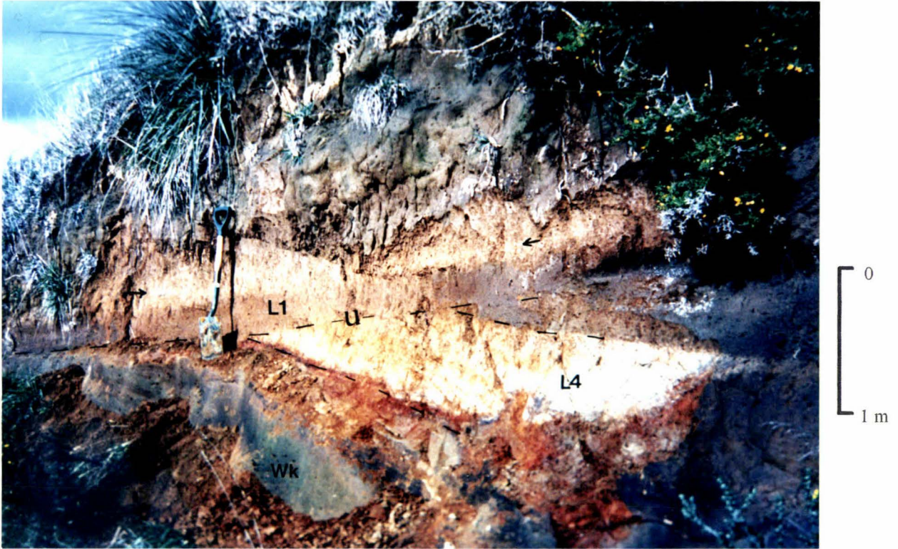
Plate 3.8 (above) Angular unconformity (-u-) on edge of Ngarino Terrace inter-fluve with L1 overlying L4 and Whakamara dunesand (Wk). Note the Kawakawa Tephra (arrows) above the unconformity. Section 16 at Q21/318718.
