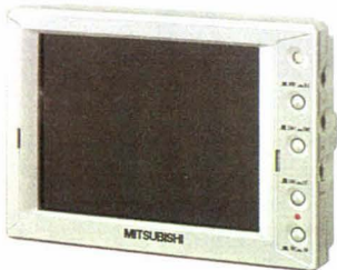
CM-7000 6.8-inch color monitor *2: PAL and NTSC dual-system
