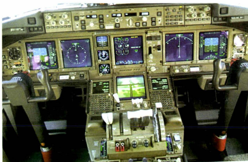
Figure 2.10 - Boeing 777 cockpit with ground manoeuvre camera system.
