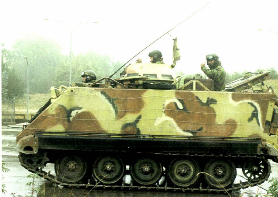
Figure 2.8 – New Zealand Army M113 vehicle with periscopes in driver's position and turret.
