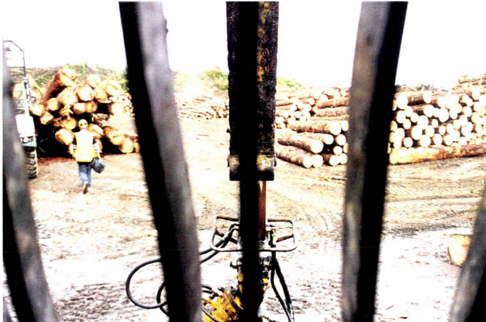
Figure 4.2 – Forward field of view of Bell Logger operator obstructed by protective bars.
