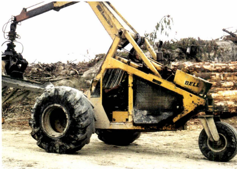
Figure 2.6 – Bell Logger forestry machine.
