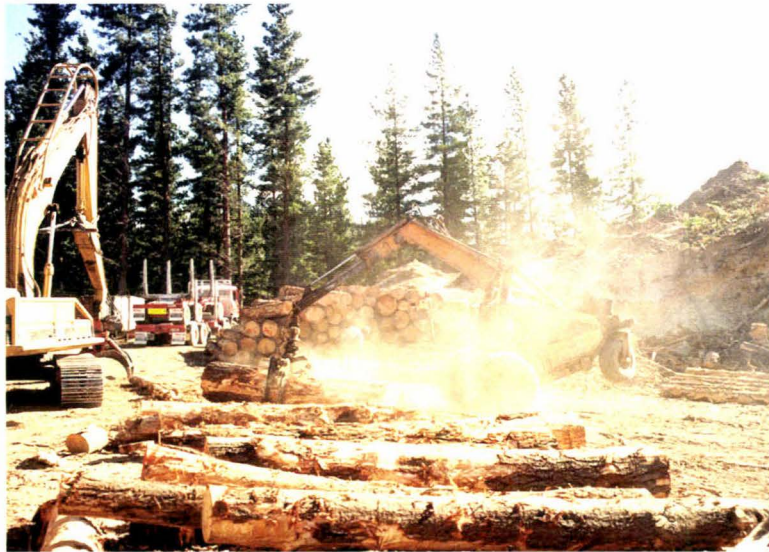
Figure 2.3 – Typical New Zealand skid site with excavator based loader (left) and Bell Logger (right).
