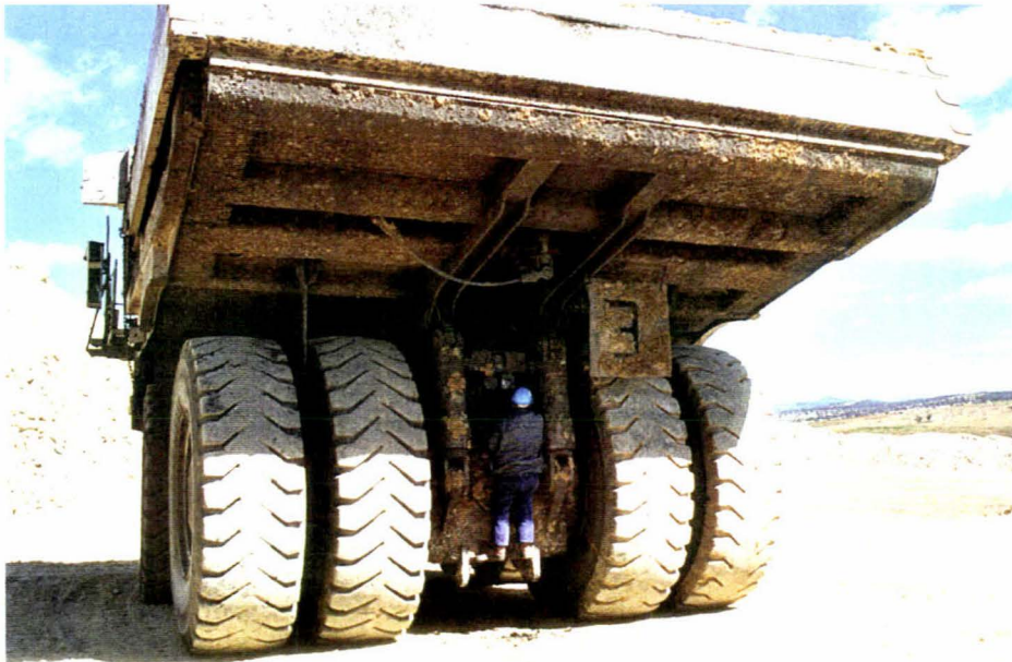
Figure 2.9 – Dump truck fitted with CSIRO rear-vision video camera “Eye in the Backside” system (operator cleaning camera lens).
