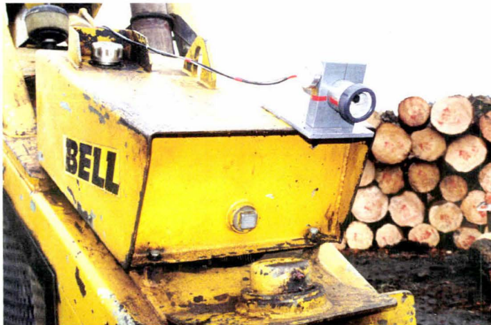
Figure 5.1 - Video camera mounted in protective metal tube on the diesel tank of the Bell Logger.
