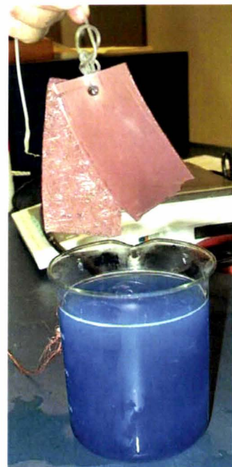
Figure 6.7-3: Colour of copper sufficiently coated copper part
