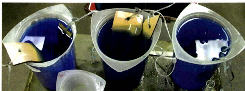
Figure 4-23: Illustration of how TEA levels affect the colour of the electroless copper solution: from left to right 5, 10 and 15 ml TEA solutions
