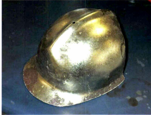
Figure 7-4: Nickel-plated UP resin sample (small construction half helmet)
