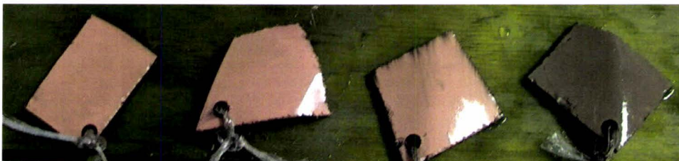
Figure 4-33: Electroless coppered samples from 5, 10, 15 and 20 ml TEA solutions consecutively. Notice colour of 4th sample is duller.
