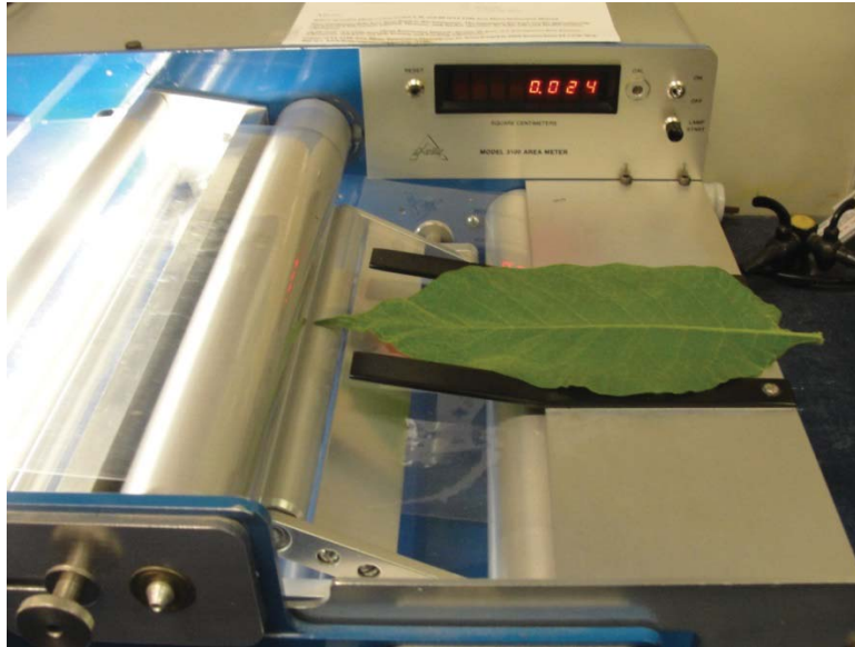
Figure 5.5. Leaf area meter used to measure woolly nightshade leaf area.
