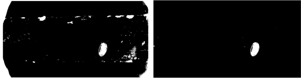
Figure 5-3, Binarized image of nematode eggs (Left: without background subtraction, Right: after background subtraction).
