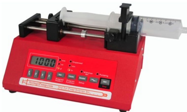
Figure 2-2, N1010 syringe pump. [40]
