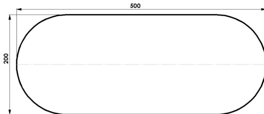
Figure 4-29, Rolled wire profile (dimensions in \mu m).
