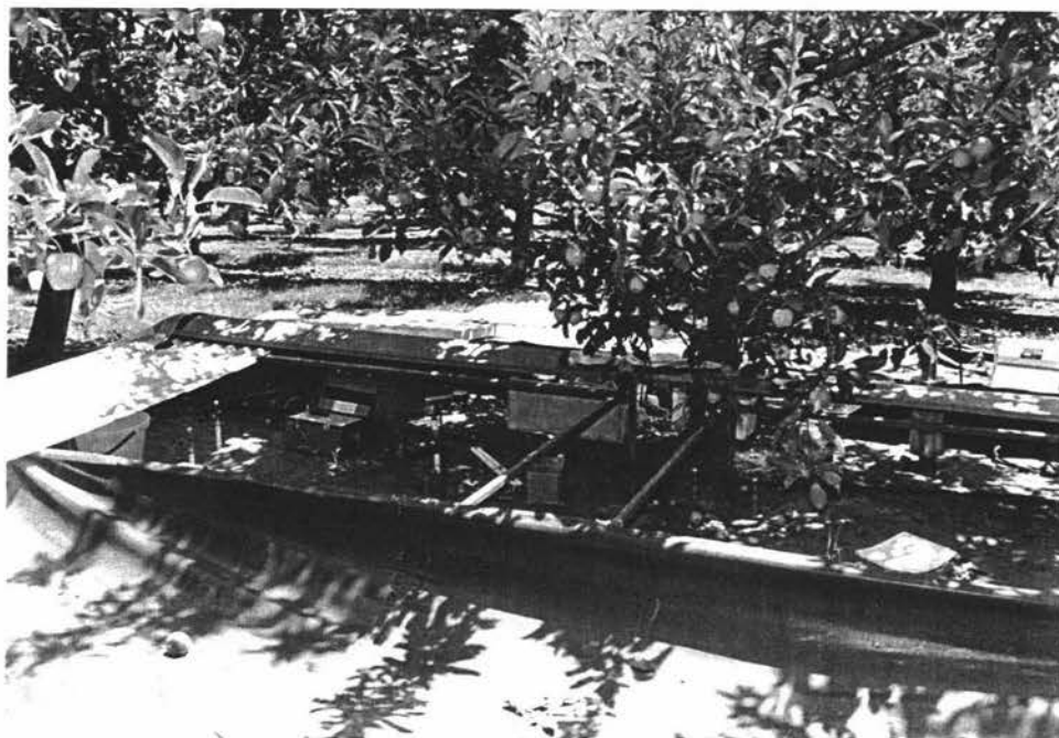
Figure 2.4. The rainout shelter around Tree U, open for measurements.
