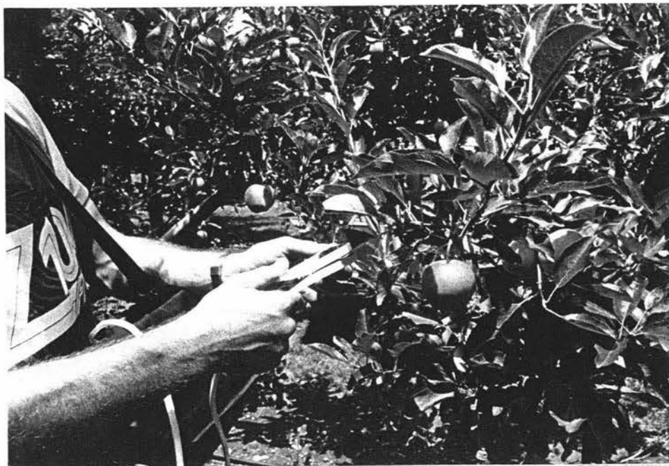
Figure 5.6(b). Using the porometer to measure the stomatal resistance of the bottom of a leaf.
