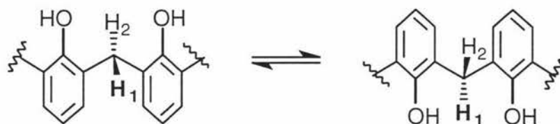
Figure 1.8. The conformational interconversion of a calixarene segment showing the different environments of the methylene protons.
