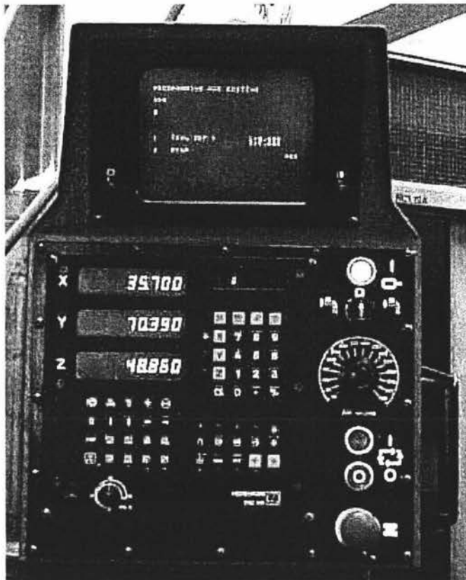
Figure 3-14 The Visual Display Unit and Pendant Control
