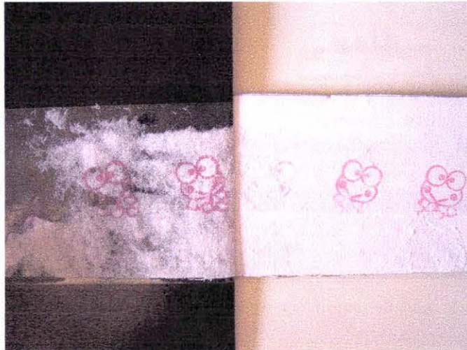
Figure 4-9 Sanrio set test specimen (right) and peeled tape substrate (left) immediate lift
