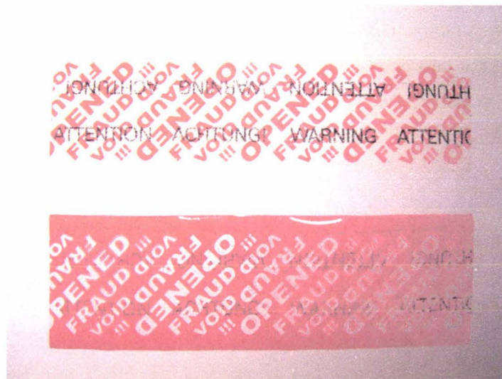
Figure 6-3 Tamper evidence tape peeled, leftover warning message (top), non adhesive top layer of tape (bottom)
