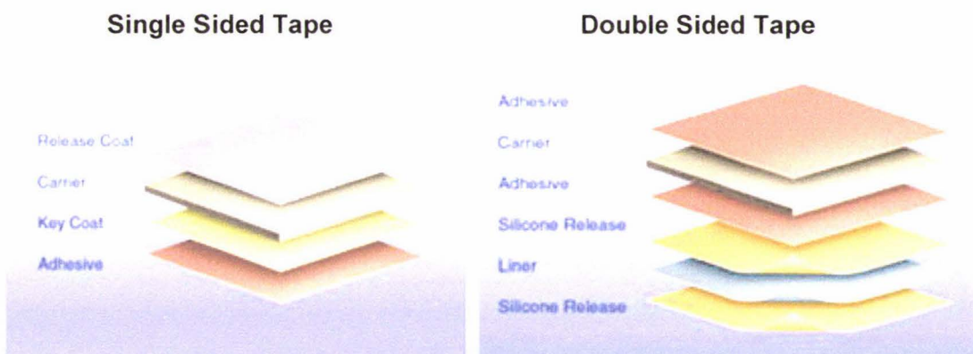
Figure 2-3 Construction of Single and Double-Sided Tape [www.sellotape.com]
