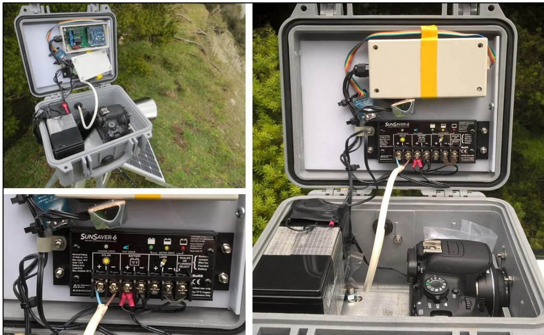
Figure 23. Time-lapse camera set-up, showing water tight casing and the solar charging panel.
