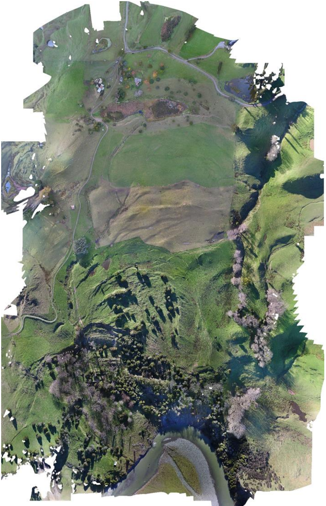
Figure 34. Orthophoto from the May 2017 photogrammetry survey, a mosaic created from the survey photos.
