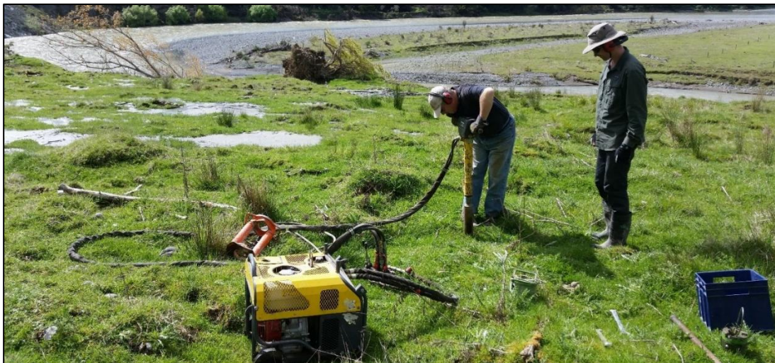
Figure 21. Photograph of the percussion corer at site 1, showing the generator (yellow), jackhammer (yellow, in use), and hydraulic jack to lift the cores back to the surface (orange). Taken on the 10 th October 2017, starring David Feek (Technician) and Sam McColl (Supervisor).
