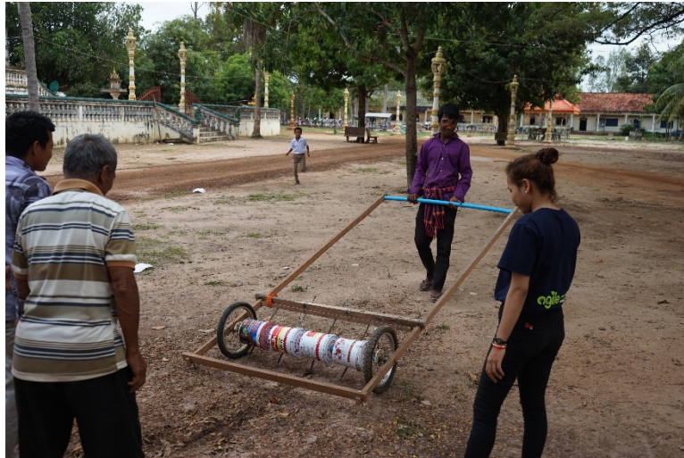
Figure 58 - Testing of community designed rice seeder
