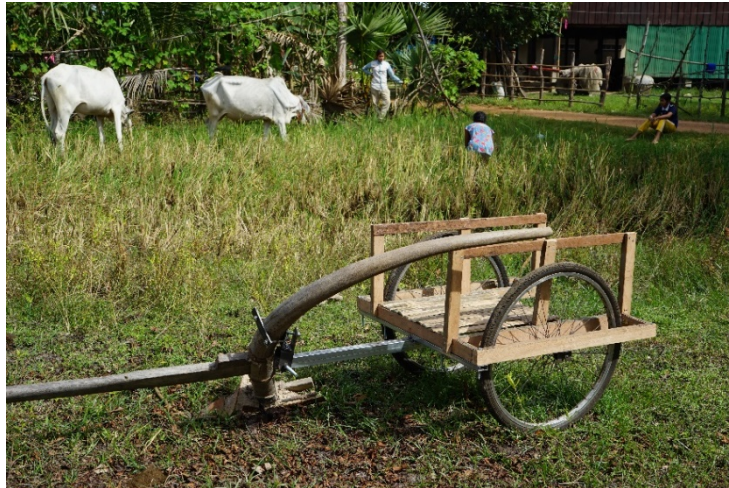
Figure 72 - Case 2 final prototype of the plough cart
