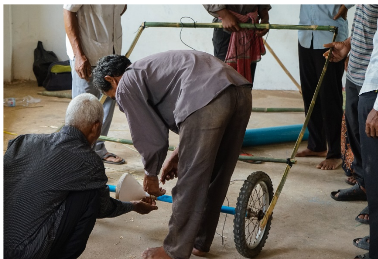
Figure 50 - Team 1 building a drum seeder prototype
