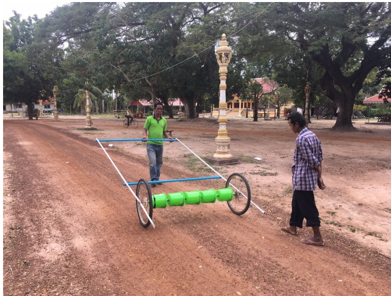
Figure 60 - Testing of D11 designed rice seeder
