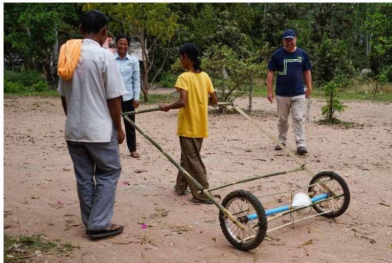
Figure 52 - Participant testing the rice seeder prototype version 2
