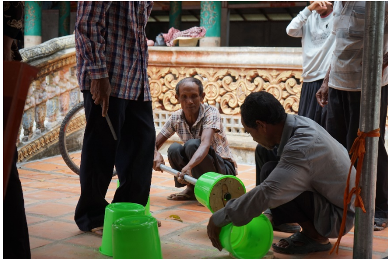
Figure 59 - Construction of D11 designed rice seeder
