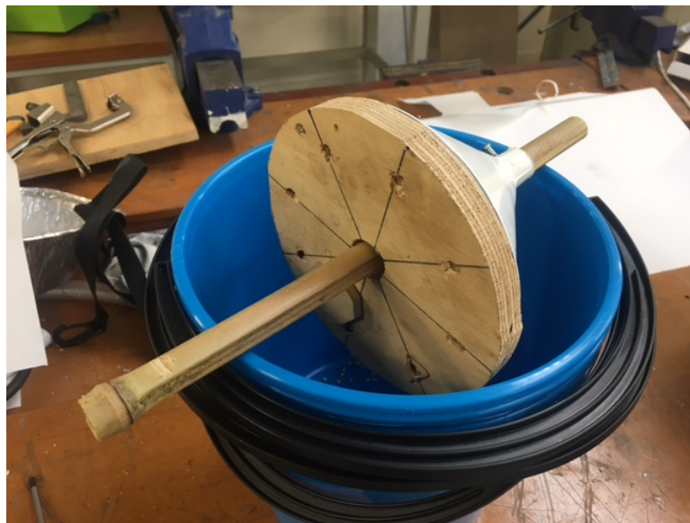
Figure 49 - Lab testing of dosing-plate for Team 1
