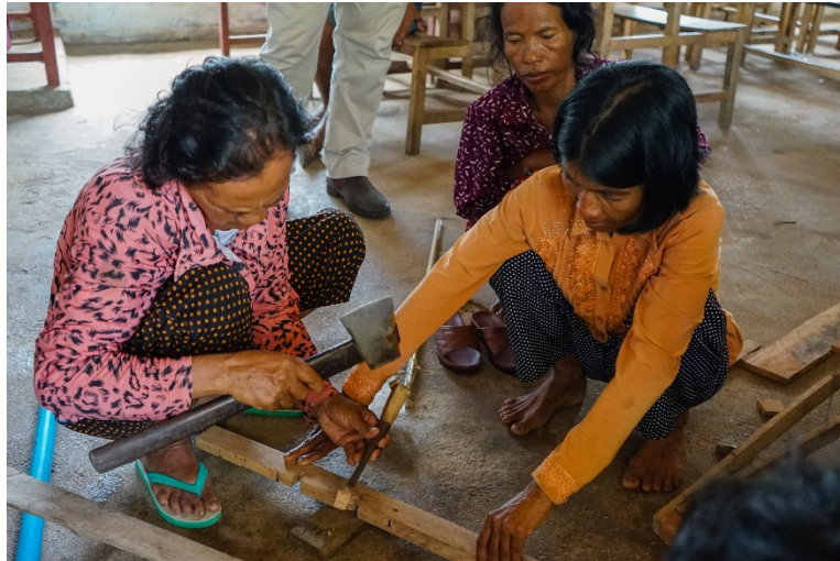
Figure 101 - Female participants notching wood for plough cart prototype in Workshop 3
