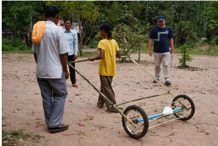
Figure 97 - Case 1 team constructing a rice seeder prototype
