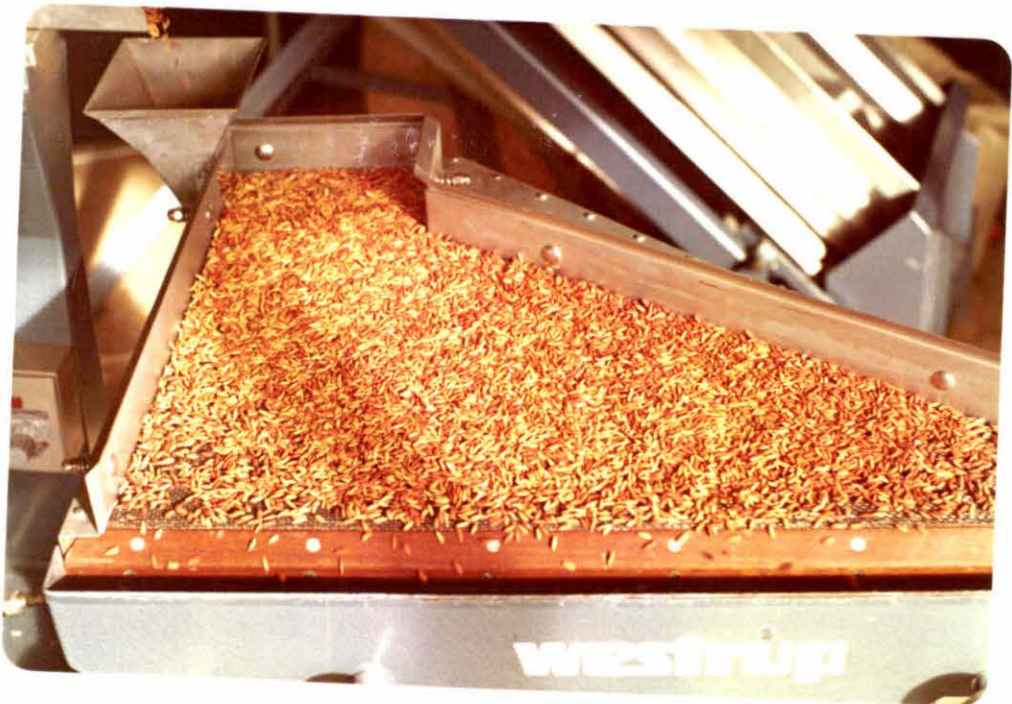
Plate 11 : Stratification and separation of seeds on a specific gravity separator
