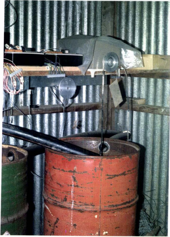
Plate 3.3 Stephens Type F water level recorder (right) and the variable potentiometer system (left) used to measure the rate at which runoff filled the 200 l drum.
