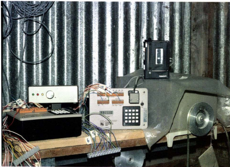
Plate 3.4 Campbell CR21 micrologger used to record automatically rainfall, runoff and water table depths.
