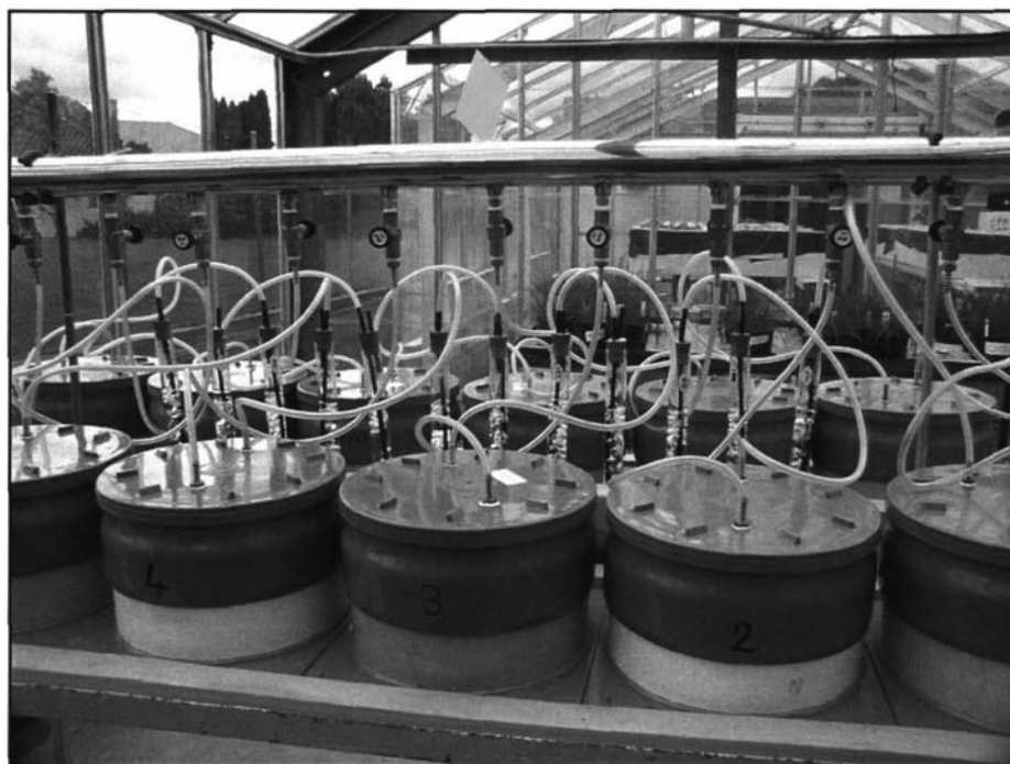
Plate 3.1 Chambers used for simultaneous measurement of \text{NH}_3 and \text{N}_2\text{O} emissions
