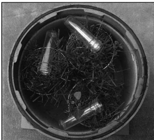
Plate 3.2 Three passive samplers placed on three cores in the chamber
