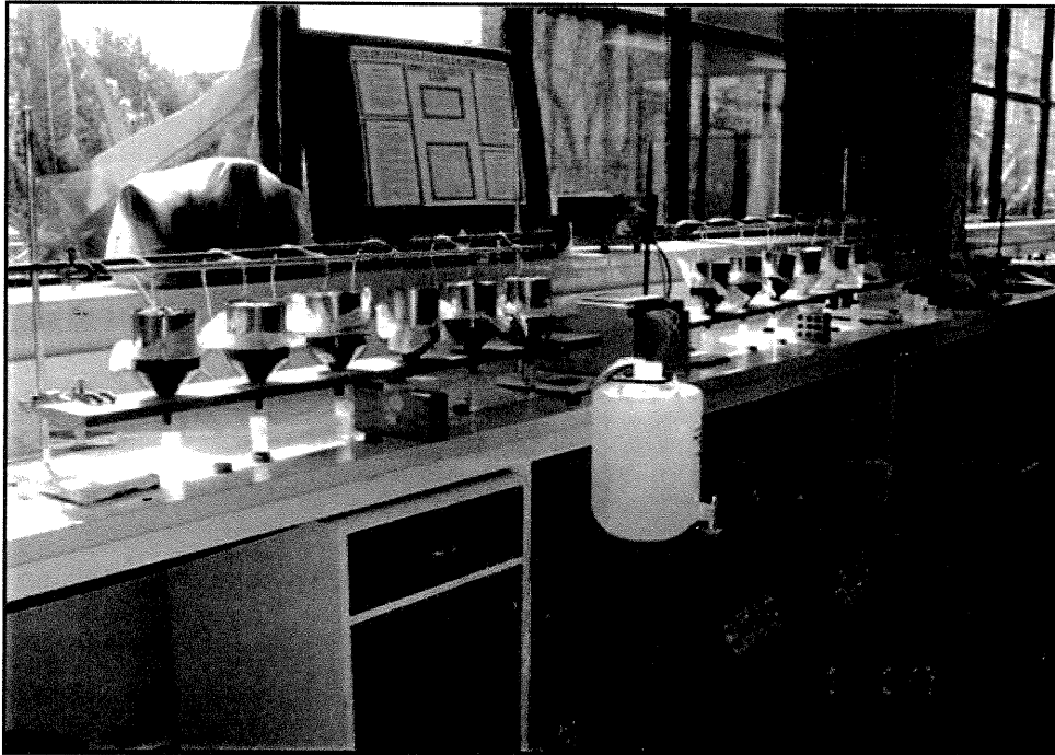
Plate 5.1 Apparatus used for leaching of soil cores.
