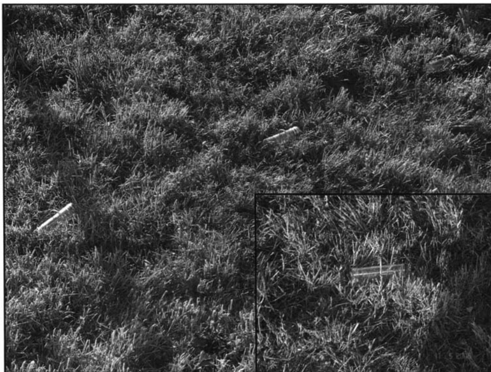
Plate 3.3 Passive samplers placed in a plot during the field-plot study
