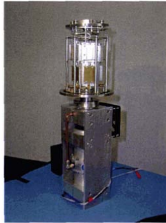
Figure 7.4. Picture of the Mast Mountable System M1 with the Dewar Open and a Full Complement of Filters
