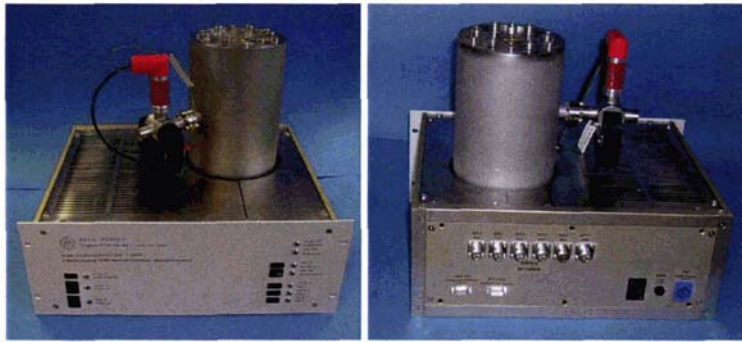
Figure 7.1. Pictures of D7 front and back showing the new N-type connectors for RF input (top of cryostat) and output (back panel)
