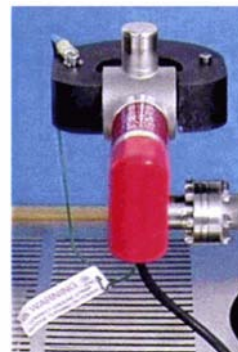
Figure 5.25. ION Getter Pump Connected to High Voltage Power Supply
