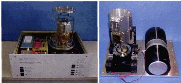
Figure 7.2. Pictures of D7 with removed cryostat enclosure to display the new obelisk with a hexagonal cross section for the mounting of 6 Filter-LNA assemblies to be used with a 3 sector CDMA base station
