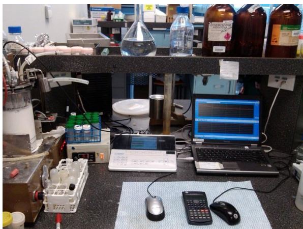
Figure 3-1 The pH-stat fermentation apparatus consisting a fermenter (left), online measuring unit (centre) and computer (right) to record and process the data.
