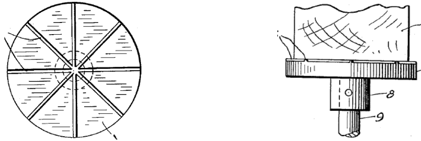
Figure 2.34: Top and side views of a flat friction wheel with grits (J et al. , 1961)
