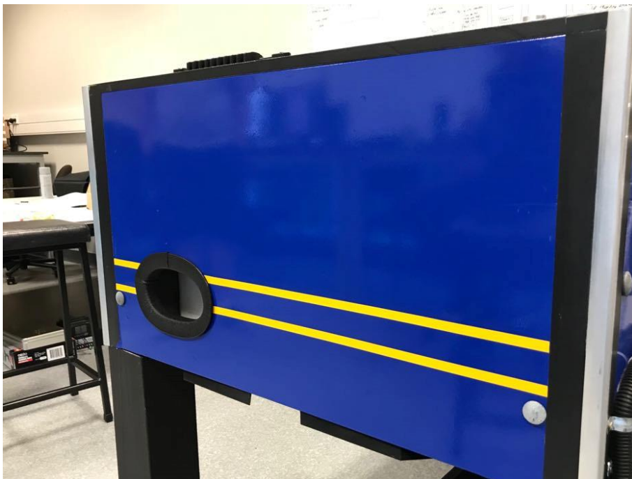
Figure 4-12 - Semi automated foosball table right hand ball return chute
