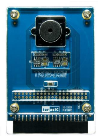
Figure 5-6 - Terasic TRDB-D5M camera development board
