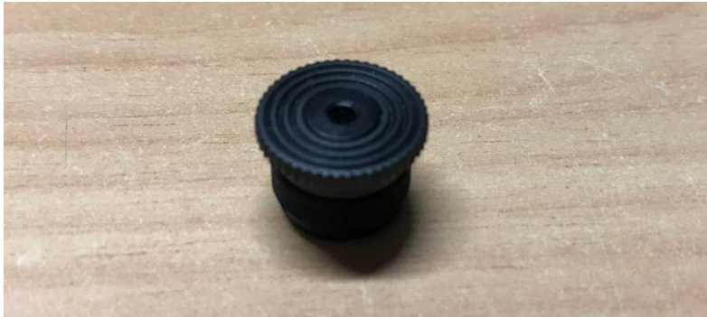
Figure 5-9 - Long focal-length (narrow angle) lens provided with the D5M camera module
