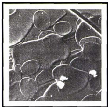
Figure 2.7: Evidence of droplet spreading and coalescence on a PVP-coated particle [taken from Link and Schlünder (1997)].
