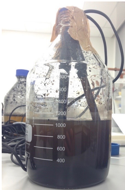
Figure 17 Experimental set up of the second scoping experiment assessing analytical techniques for measuring nutrient uptake capacity of lignite slurry versus raw, un-sieved lignite: Sample A with pH and conductivity probe.
