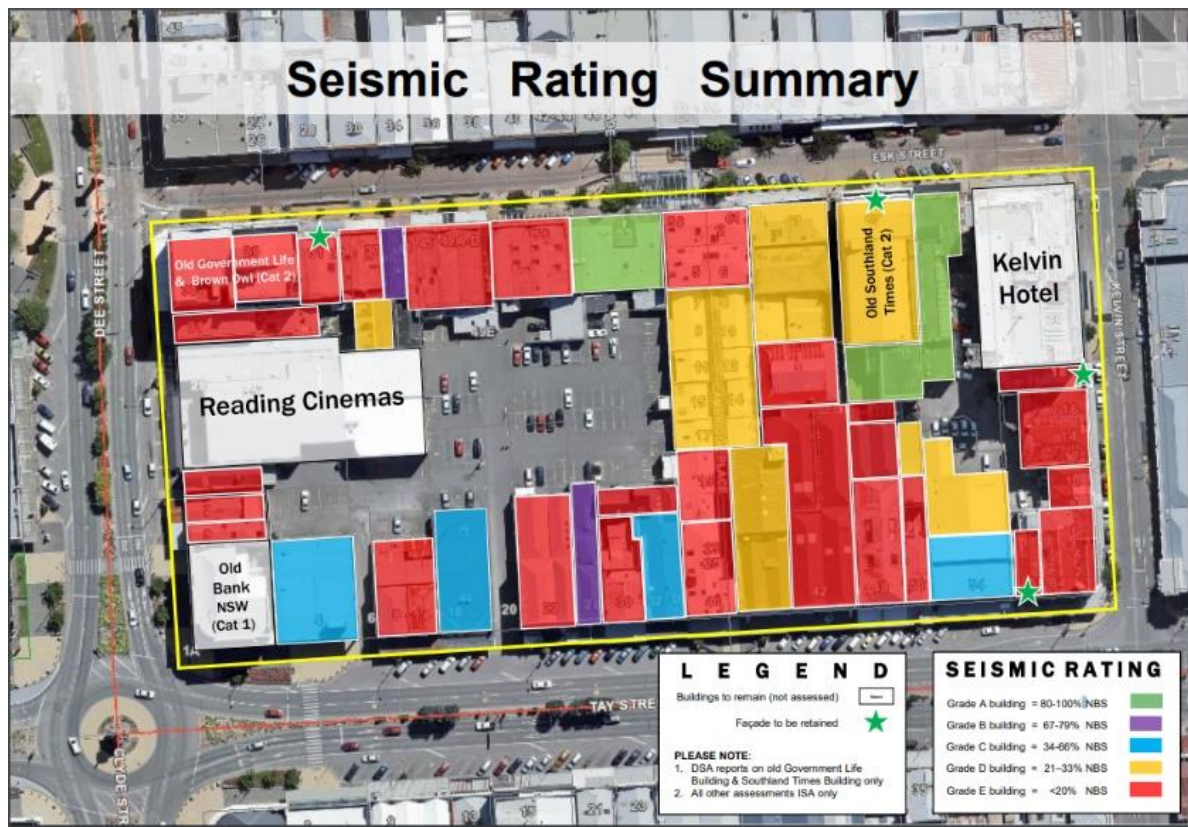
Figure 4.9: Seismic rating summary of HWCP inner-city redevelopment block. Source: (McDougall & Marriott, 2019)
