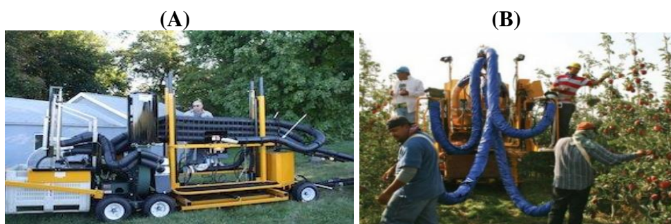
Figure 3.11. Pneumatic vacuum apple harvesters: DBR (A) and Oxbo (B) Sources: Warner (2012) and Lehnert (2012).
