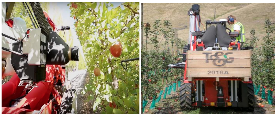
Figure 3.2. Robotic apple harvester with suction mechanism (Commercially trialled) Sources: Dininny and Mullinax (2016) and Chumko (2019).
