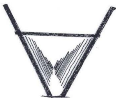
Figure 3.17. V-shaped canopy system Source: Apples and Pears Australia Ltd. (2012).
