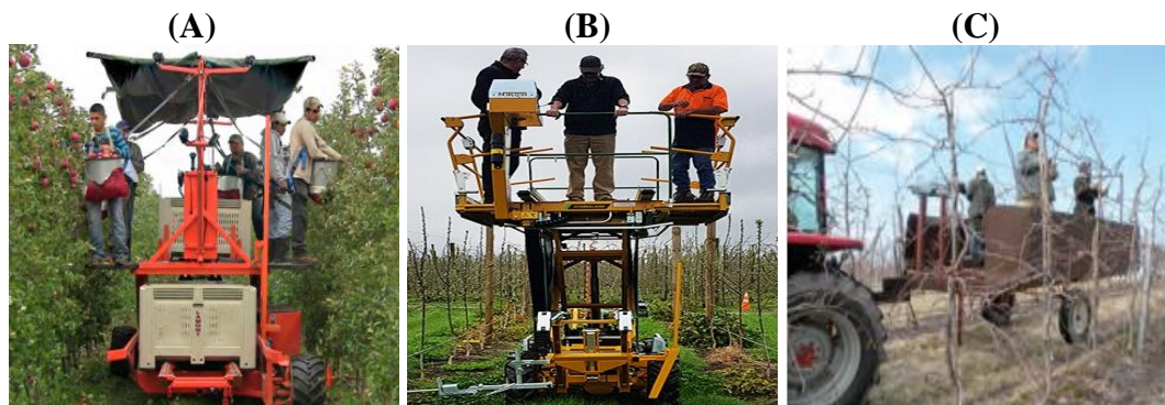
Figure 3.9. Orchard platform types: Self-propelled single-level (A) and multi-level (B), and tractor pulled (C). Sources: Sazo et al. (2010), Wells et al. (2017b), and Hydralada (2018).
