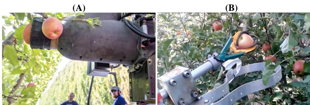
Figure 3.8. Robotic apple harvester types: suction (A) and gripper (B) mechanisms. Sources: Dinunny and Mullinax (2016) and Dinunny (2017).
