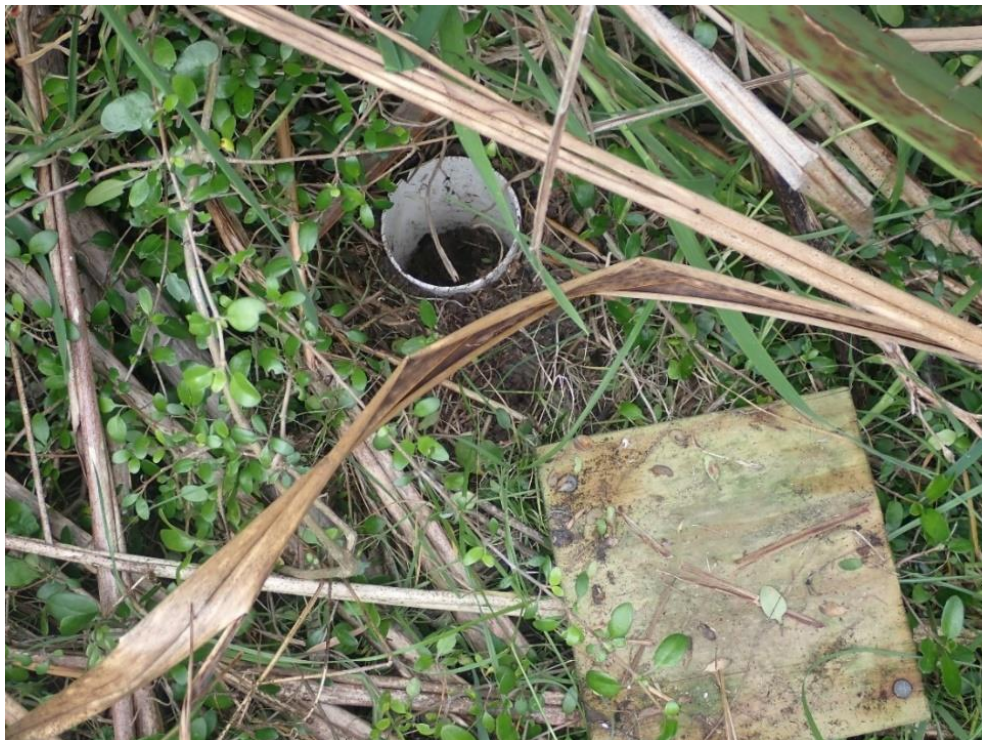
Figure 17. A small pitfall trap disassembled, showing the downpipe into which a small cup of ethanol is placed to complete the arming process. This was then covered by the wooden lid shown in the bottom right. Photo: W. Brockelsby, Mana Island, October 2021, CC-BY.
