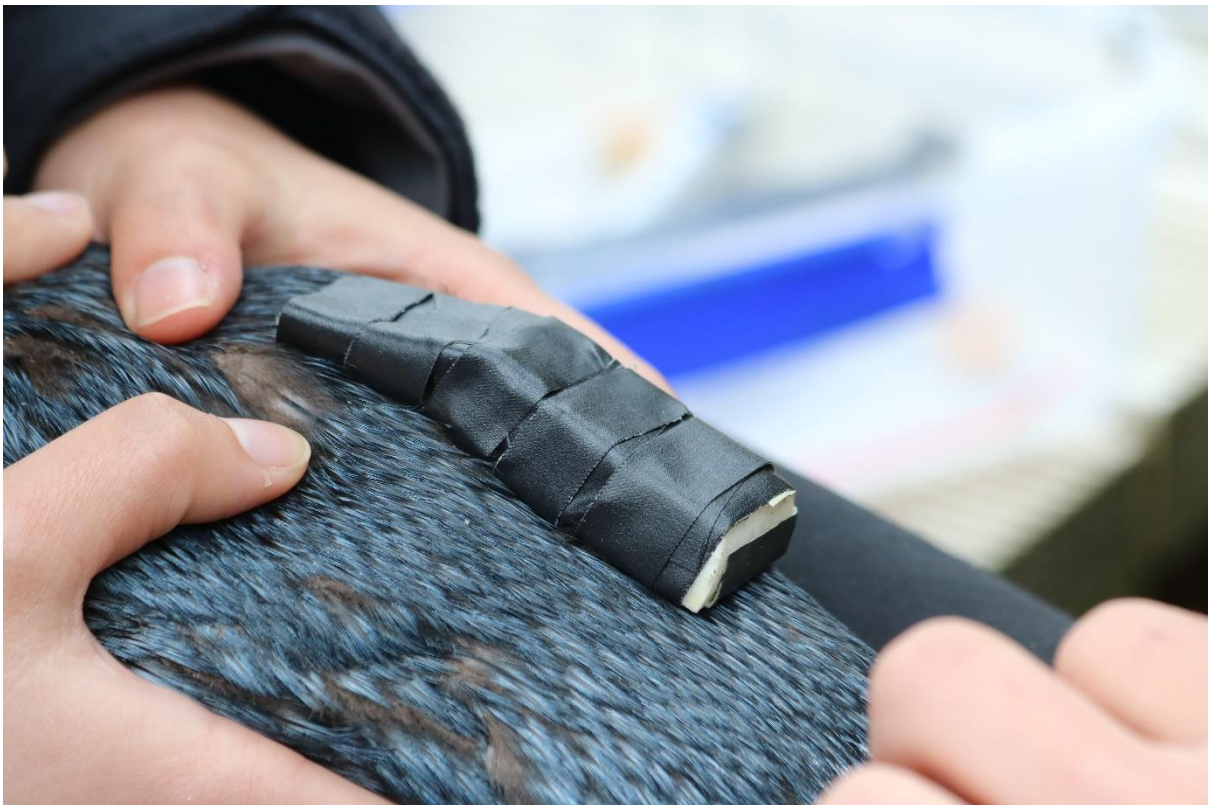
Fig. 2.2. An Axy-Trek device attached to a penguin. Tape was wrapped around the device and the underside of the feathers. An additional triangular piece was attached at the front to further streamline the device and reduce the chance of device loss when moving in and out of the nestbox.
