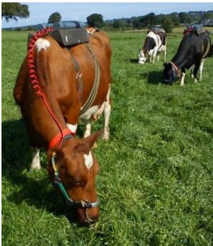
Figure 2.4. \text{SF}_6 tracer technique on a grazing dairy cow at Teagasc Moorepark, Ireland (Berndt et al. 2014)
