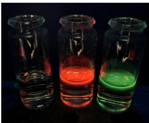
Figure 30. [ La(L 1 ) 3 ] 3- (left), [ Eu(L 1 ) 3 ] 3- (middle) and [ Tb(L 1 ) 3 ] 3- (right) in H 2 O ( 1 \times 10^{-3} M) under short wave UV light
