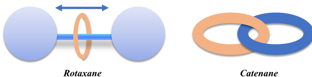
Figure 11. Schematic showing the interlocked nature of the rotaxane and catenane
