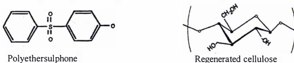
Fig. 4.7 Structures of polyethersulphone and regenerated cellulose (Cheryan 1998)
