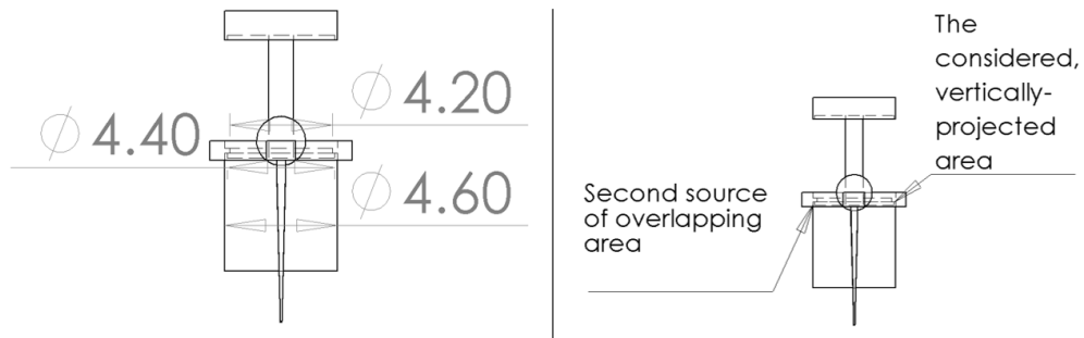
Figure 3.36: The ridges added to the centre-pin served to keep overlapping area small, and increase vertical separation. However, the size of the outer cut-out on the lever arm was the same diameter as the outside of the pin, meaning that “cupping” of the centre pin during settling would actually increase the contact area between parts.
