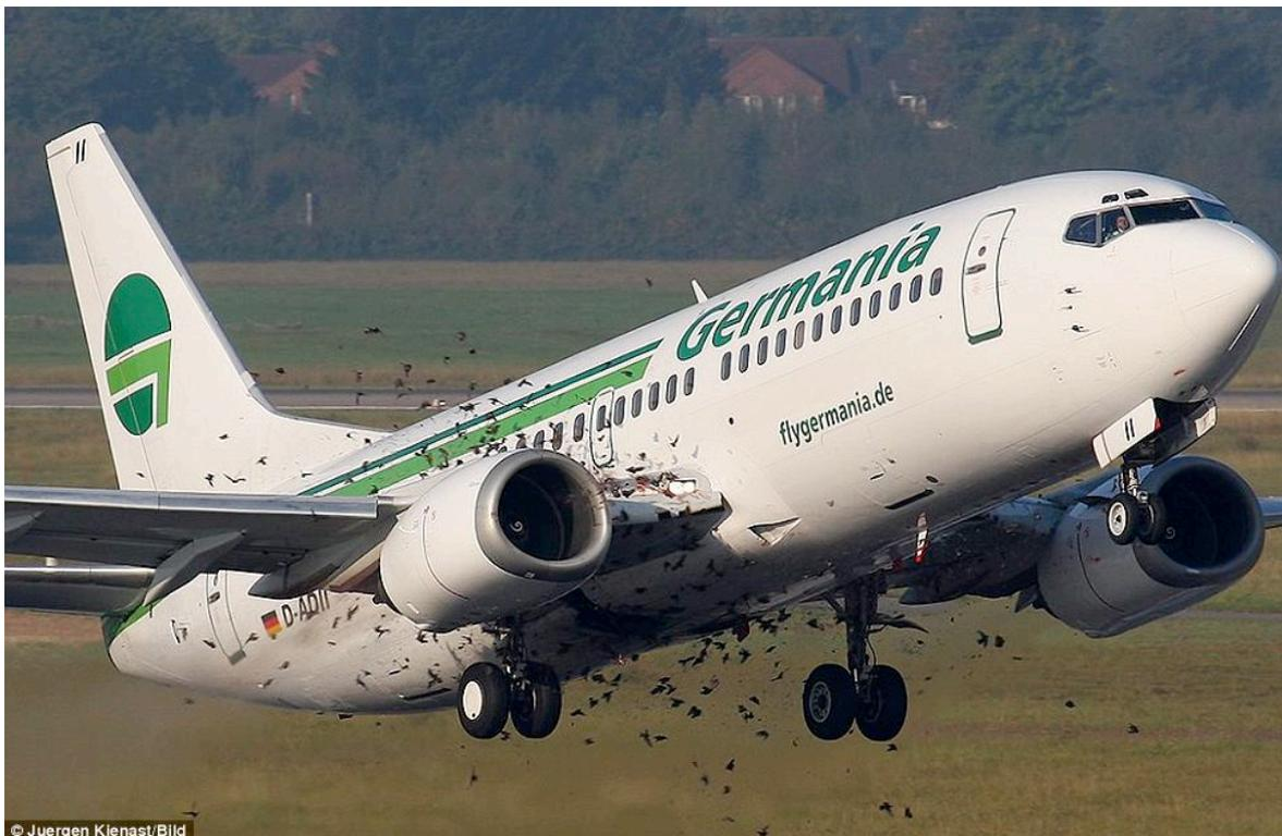
**Figure 6.1** This Boeing 737 passenger jet struck a flock of more than 200 starlings while climbing after takeoff from Düsseldorf airport in Germany in October 2009. It returned and made a safe landing back at Düsseldorf on one engine 45 minutes later. The cost of repairs exceeded \$US1 000 000. (Photograph Juergen Kienast)
