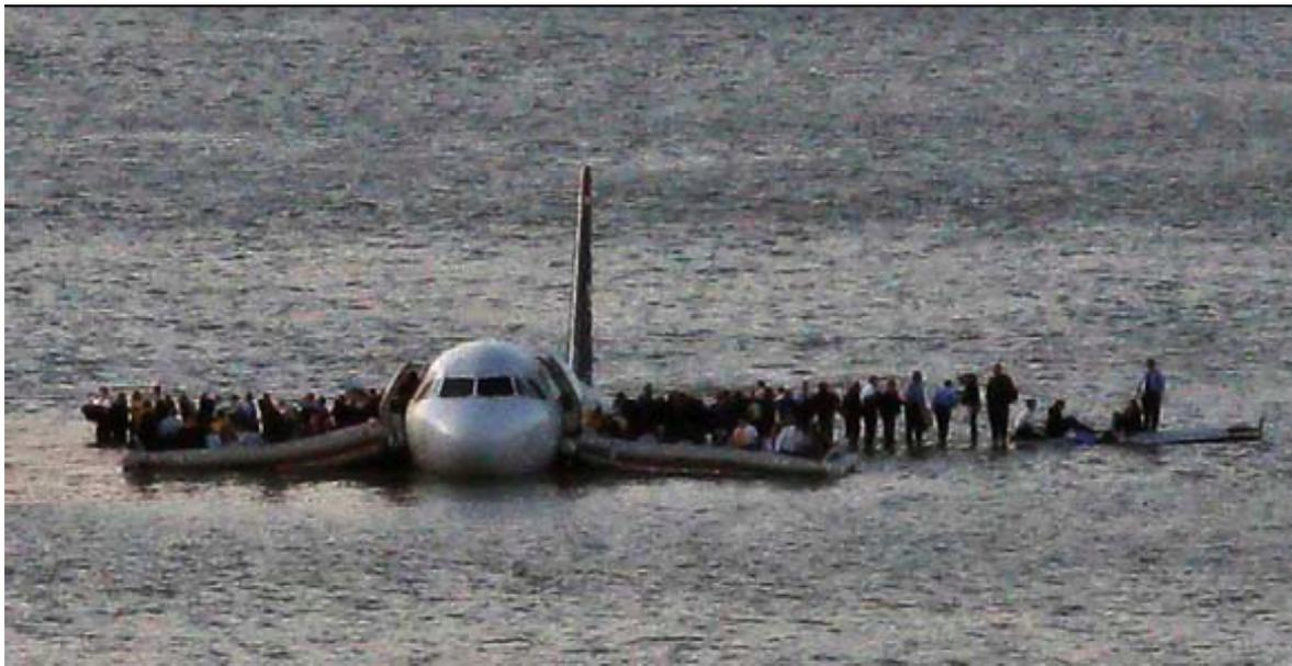
**Figure 6.6** US Airways Airbus 320 flight 1549 after making a forced landing in the Hudson River on 15 January 2009. The aircraft suffered a multiple ingestion of Canada geese into both engines with a resultant complete loss of power. All passengers and crew survived. The aircraft was a total loss at a cost of \$US55-65 million. (Photo Associated Press)<sup>[14]</sup>
