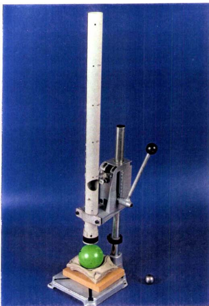
Fig. 3.1 Apparatus used to apply a standard bruise to individual apples using a 25 mm diameter steel ball.
