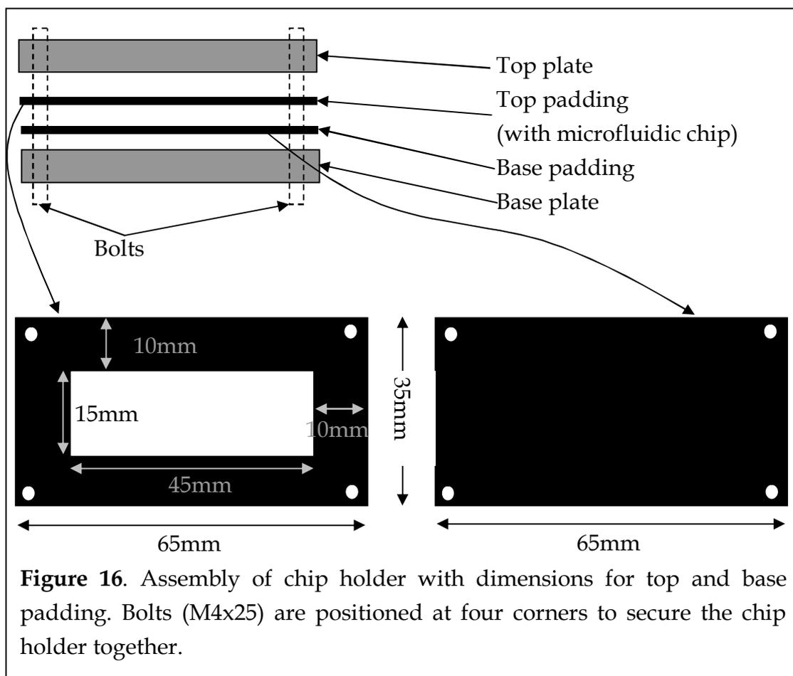
**Figure 16.** Assembly of chip holder with dimensions for top and base padding. Bolts (M4x25) are positioned at four corners to secure the chip holder together.
