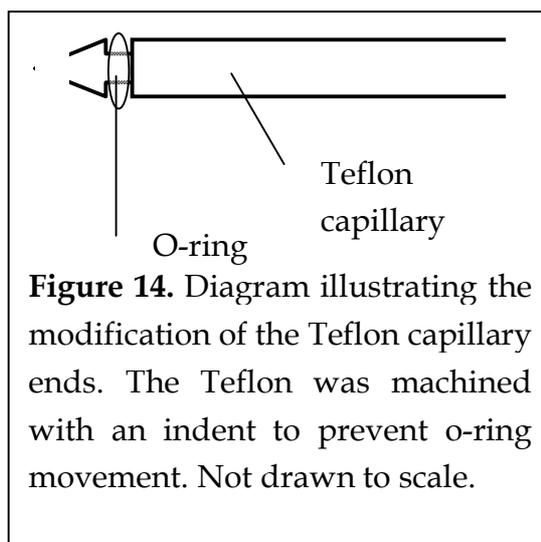
**Figure 14.** Diagram illustrating the modification of the Teflon capillary ends. The Teflon was machined with an indent to prevent o-ring movement. Not drawn to scale.
