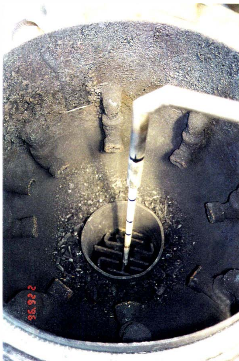
Figure 5.5 Position of the high temperature probe in the gasifier
