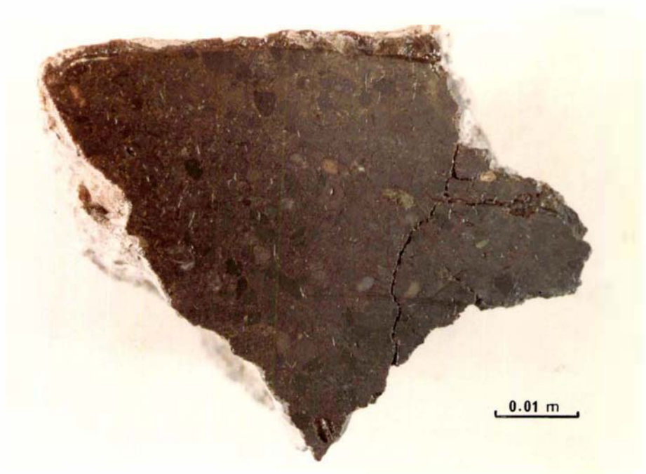
FIGURE 2.4: Coarser sized pebbles than in Figure 2.3 set within a medium-grained sandstone matrix. Note the rounded to subangular shape of the constituent pebbles. Rock sample Mte5 from Mangatera foothills area at locality U23/735188.
