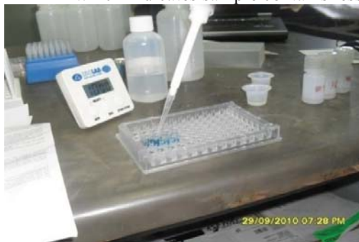
Photo 3: Alert test kit sample interpretation. Sample shows a darker blue colour than the control which indicates sample contains less than 10 ppm of histamine.
