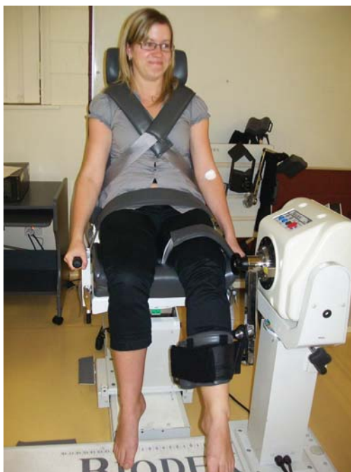
Figure 6 Participant completing 5 maximal eccentric repetitions of the quadriceps muscle on the Biodex isokinetic dynamometer. The same eccentric motion was carried out for the damage protocol
