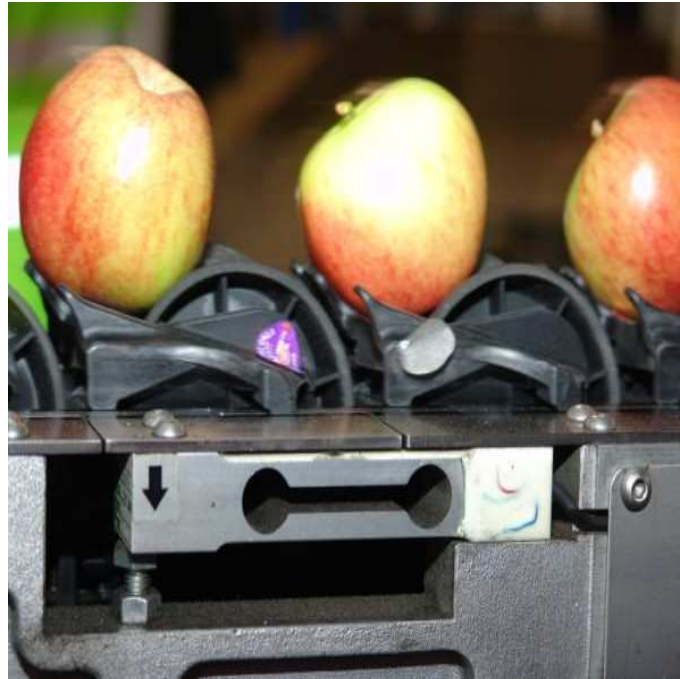
Figure 3: Apples on a Vishay Load Cell
