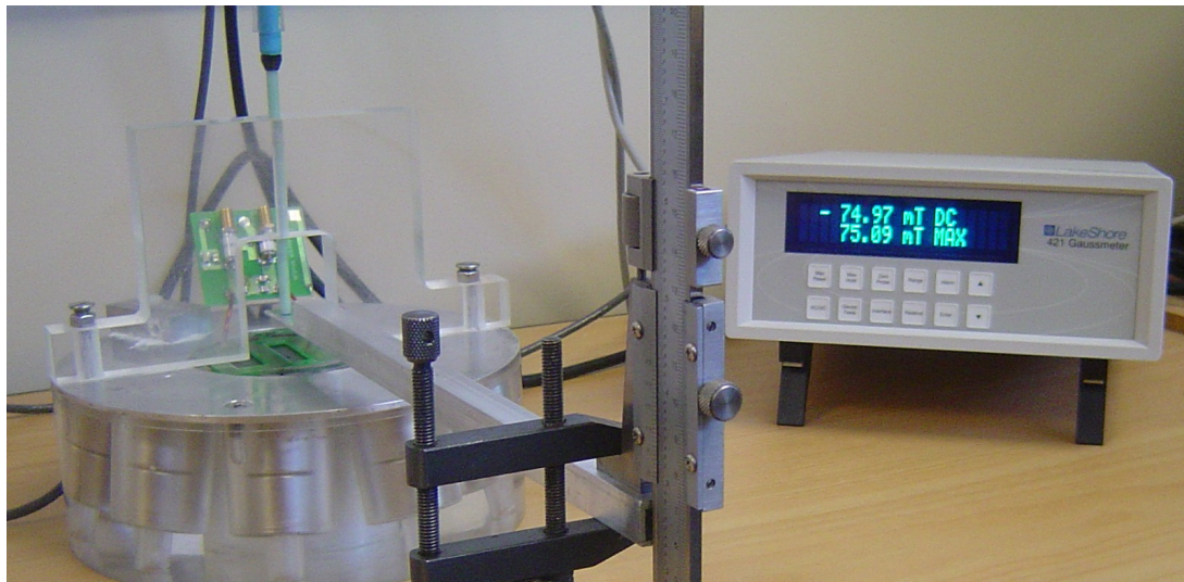
Figure 2.16: Measuring the B_0 field profile using a Hall effect probe. The probe was positioned vertically with the aid of a Perspex jig. A Vernier height gauge used for the height measurements had an aluminium arm clamped onto it to keep the metal gauge at a distance from the magnet.
