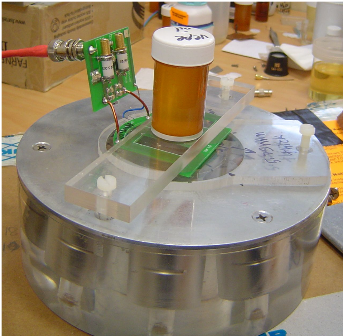
Figure 2.2: The Mole probe and tune/match circuitry used for most of this project. This is not the original Mole probe supplied for this project as will be discussed in the text. Sample vials and Perspex vial holders are discussed in §2.4.9 on page 52. Some of the NIB magnets can be seen located in pairs inside the Mole’s Perspex former. The lone central magnet is located beneath the sample vial and B_1 coil.
