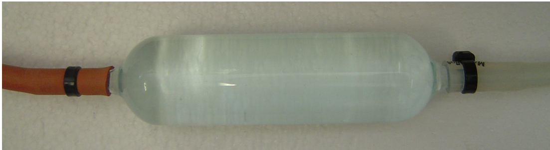
Figure 6.1: Glass flow tube and attached piping. The inside diameter of the body of the glass tube was around 31mm and the inside diameter of the two ends around 4mm. The larger diameter was constant over a length of about 95mm.
