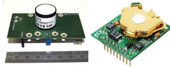
Figure 3-17: Non-dispersive Infrared CO 2 Sensors
