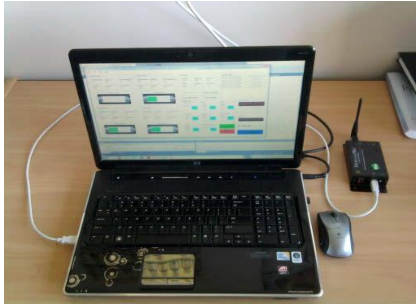
Figure 5-35: Final design of the central station
