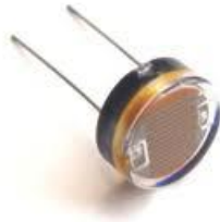
Figure 3-23: NORP12 light dependent resistor
