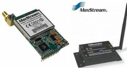
Figure 5-5: 2.4 GHz XStream-PKG RF modem
