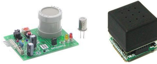
Figure 3-16: Electrochemical CO 2 Sensors
