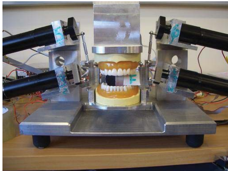
Figure 3.3 The 6RSS robot after modification
