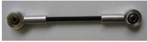
Figure 2.11 The coupler with spherical rod ends (Pap 2005)
