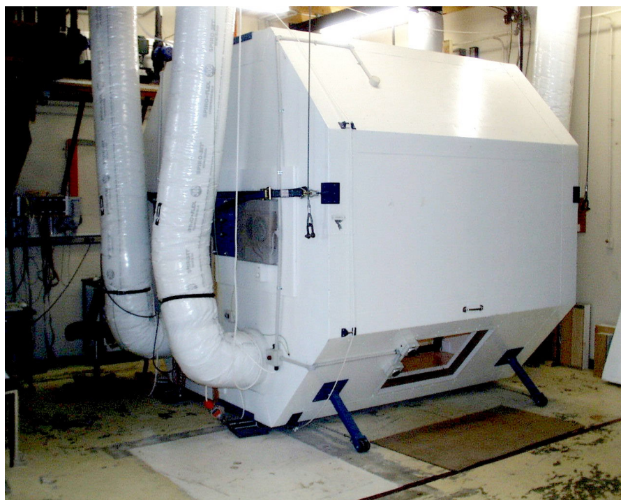
Figure C.2 Guarded Rotatable Hotbox
