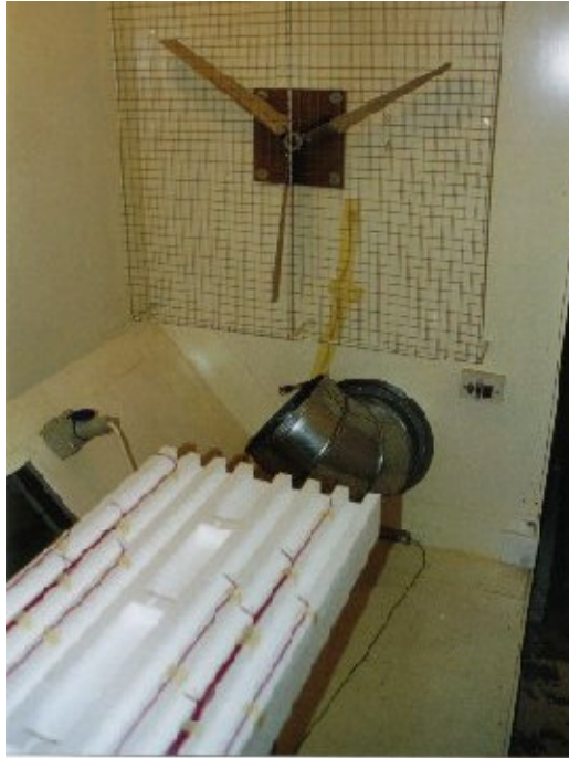
Figure C.7 Inside of Guarded Rotatable Hotbox with base relocated to the centre of the chamber
