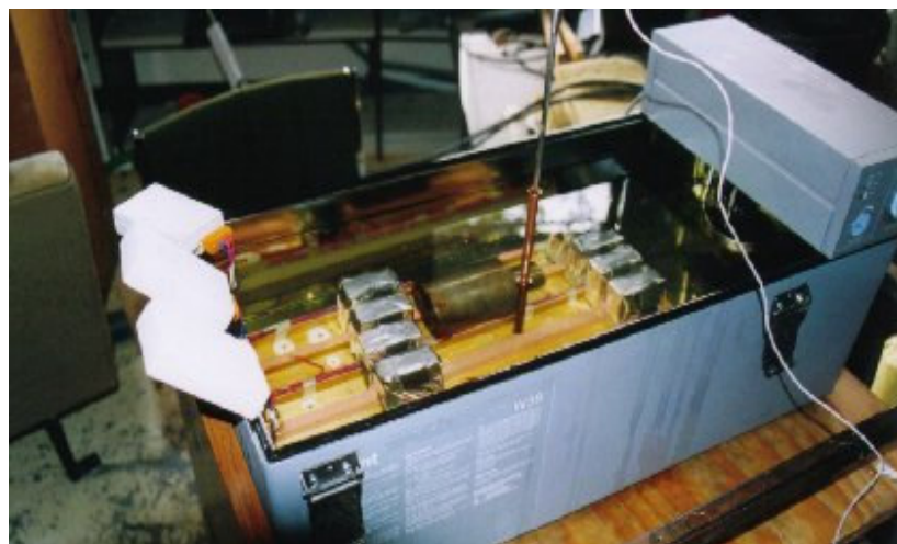
Figure C.1 Oil calibration bath
