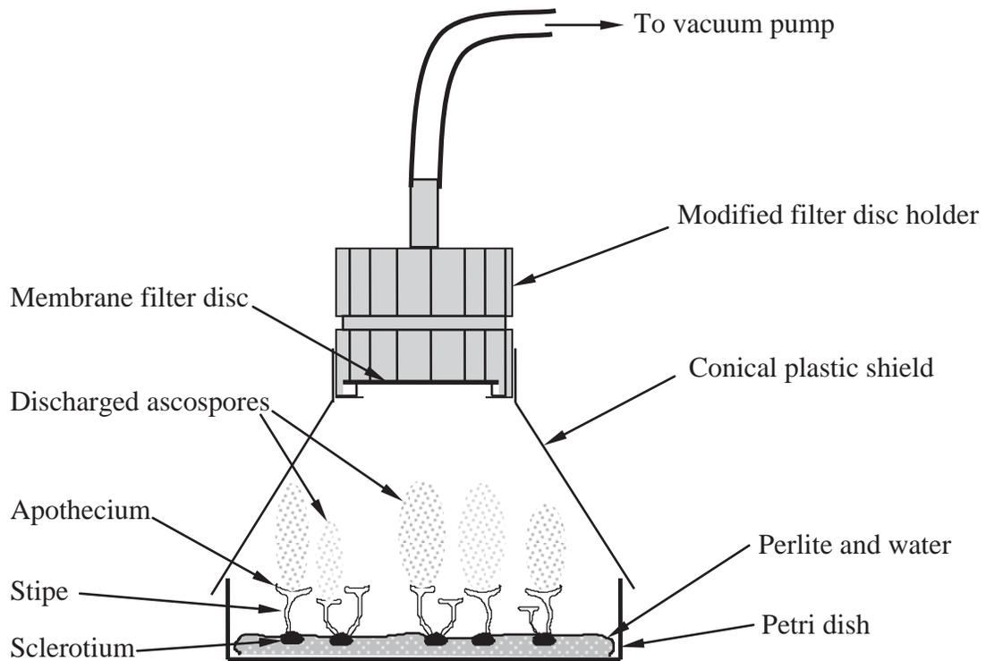
**Modified membrane filter disc holder with conical plastic shield connected to vacuum pump, and Petri dish with mature apothecia discharging ascospores.**
