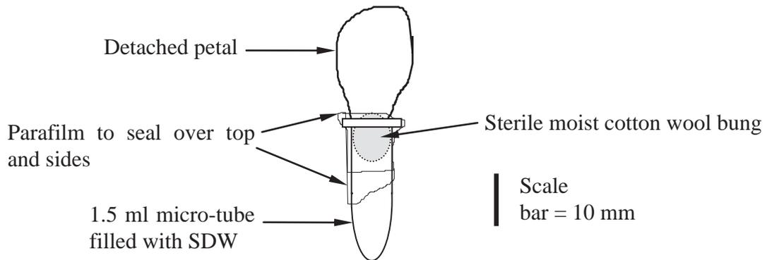
**Figure 4.2 Micro-tube holder: kiwifruit petal supported within a micro-tube by means of a cotton wool bung and parafilm.**
