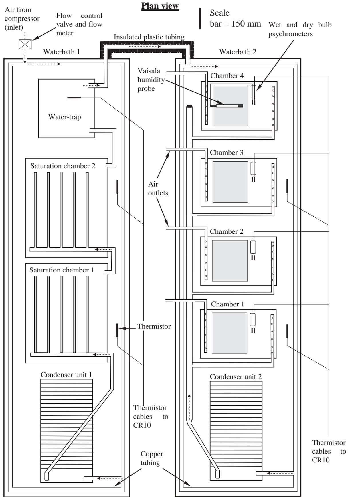
Figure 4.4 Schematic diagram of controlled environment chambers constructed within two large waterbaths, ( ..... → = direction of air flow).
