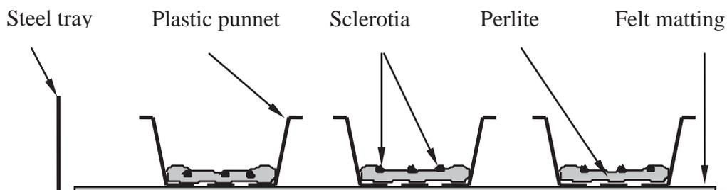
**Cross-section of plastic punnets containing Perlite and sclerotia on felt matting inside a steel tray used for induction of stipes at 4–6°C.**
