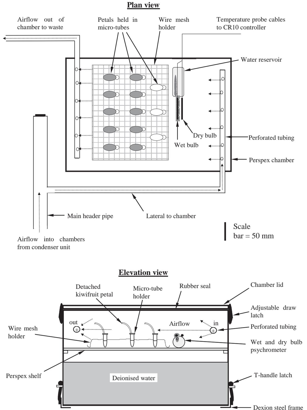
**Figure 4.5** Schematic diagram of an individual controlled environment incubation chamber in waterbath 2, showing air flow (.....→), position of petals in micro-tubes and wet- and dry-bulb thermistors.
