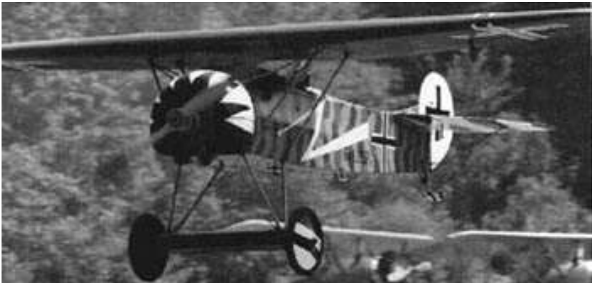
Figure 20: Fokker DVIII , a modern parasol design that was only just reaching front-line service by the time of the Armistice. Source: www.theaerodrome.com
