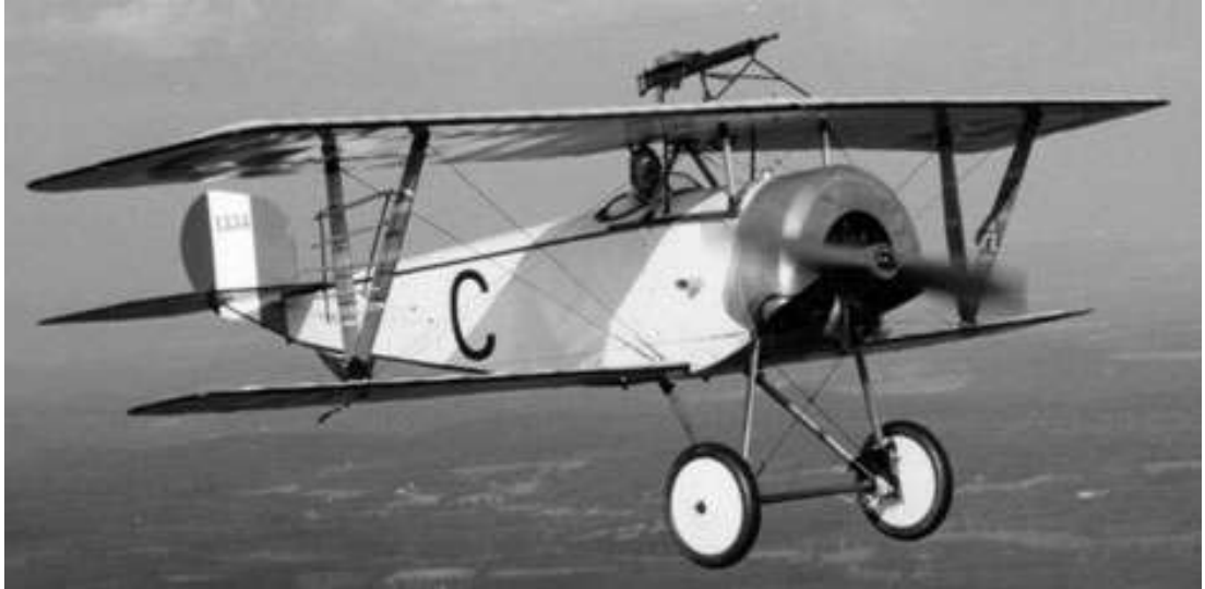
Figure 8: Nieuport N.11 , an early model of a successful French line of fighter aircraft that would see service throughout the war in both French and RFC service. Source: www.theaerodrome.com
