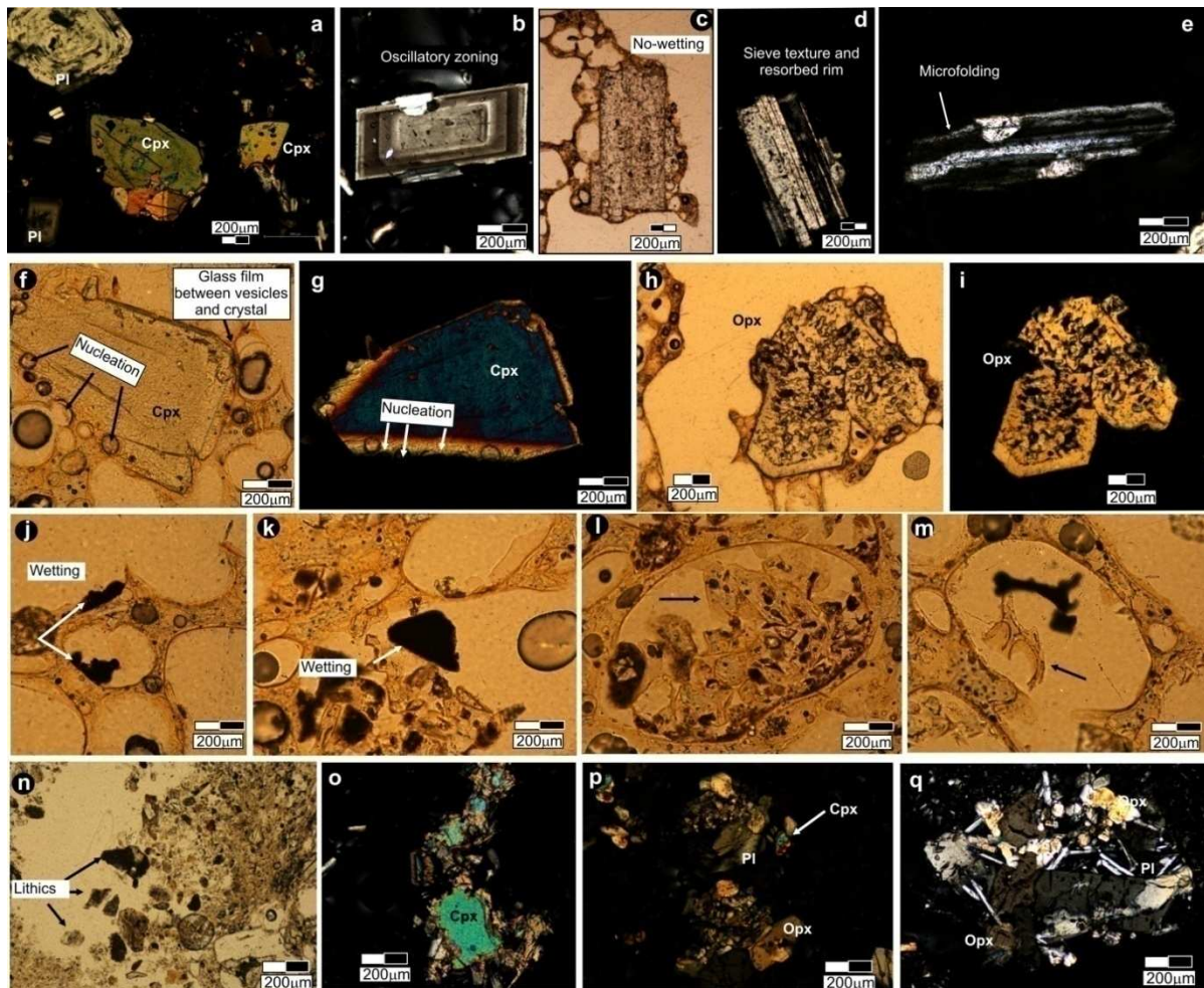
Figure 5.5 Main crystal phases in the Mgt unit (a). Plagioclase phenocrysts are commonly euhedral, zoned (b), subhedral sieved (c, d), an occasionally show plastic micro-deformation (e). Clinopyroxenes are commonly subhedral to anhedral and occasionally show “bubble wall-texture” (f, g). Orthopyroxenes (h, i) are commonly euhedral to subhedral, sieved, and vesicles do not seem to wet the crystal. Oxides are commonly embedded within vesicles (j, k). Vesicles embedding pumice fragments (l) or glass shards (m) are common. Non juvenile fragments are mainly volcanic aphanitic (n) or microphaneritic andesites (o-q).
