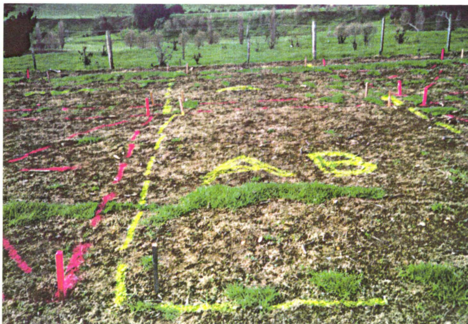
Photograph 4.10: Construction of the Ashhurst trial: the trial has been sprayed with herbicide, pegged out and treatments identified with fluorescent paint.
