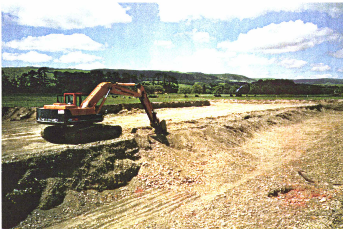
Photograph 4.8: Commercial extraction of aggregate adjacent to the Rangitikei trial site. The sandy overburden has been removed and a hydraulic excavator is removing the first cut of aggregate.
