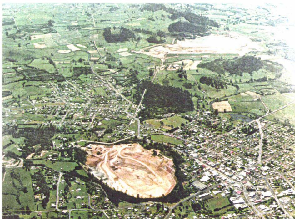
Photograph 3.5: The Waihi Gold Mining Company mine. The pit, at bottom centre, is linked by a conveyor belt to the processing plant and the tailings dam at top right.
