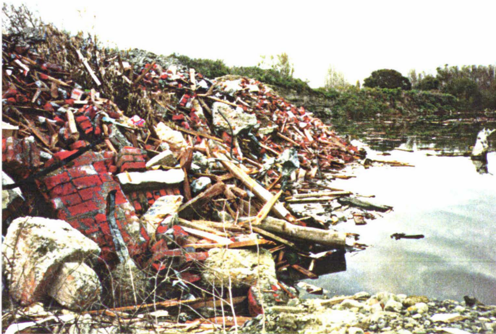
Photograph 4.4: A fill area adjacent to the Rangitikei trial site. Note the variety of organic and inorganic materials. Similar materials were used as fill at the trial site.
