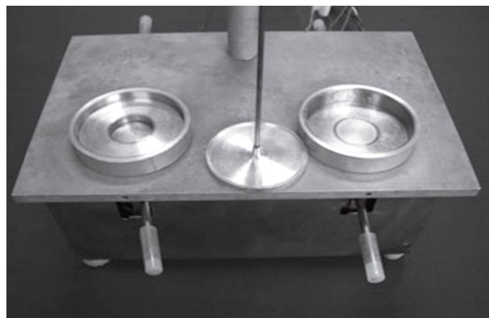
Figure 10 Schematic diagram of the UW melt meter, a modified squeezing flow test device: A/D = analog-to-digital converter; LVDT = linear variable differential transformer(Wang et al., 1998).
