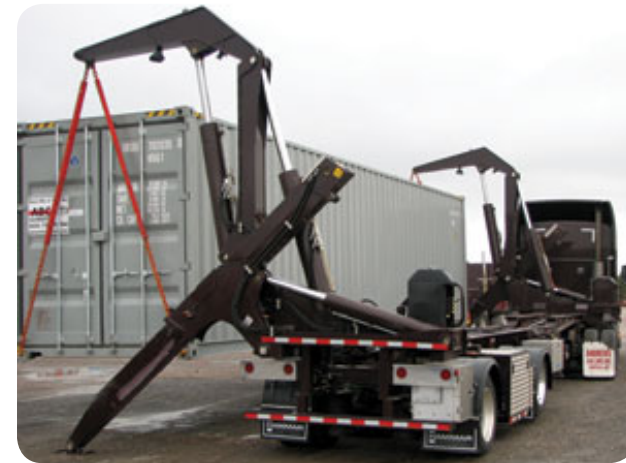
Figure 36. A HIAB truck off loading a 12 metre shipping container, Manakau, NZ.
