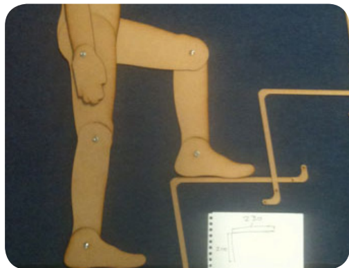
Figure 87. Using the model to establish a maximum stair riser height (220mm) and a minimum tread depth (230mm).
